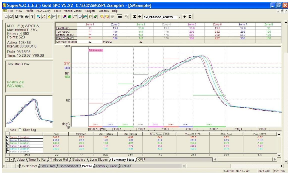
Figure 21 – Reflow Cycle (Profile)
