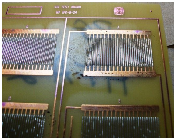
Figure 18 – Pizza Grease with Reflowed Solder Paste
