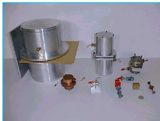
Figure 2 – LCP samples supplied and examples of cavities used for the characterization
