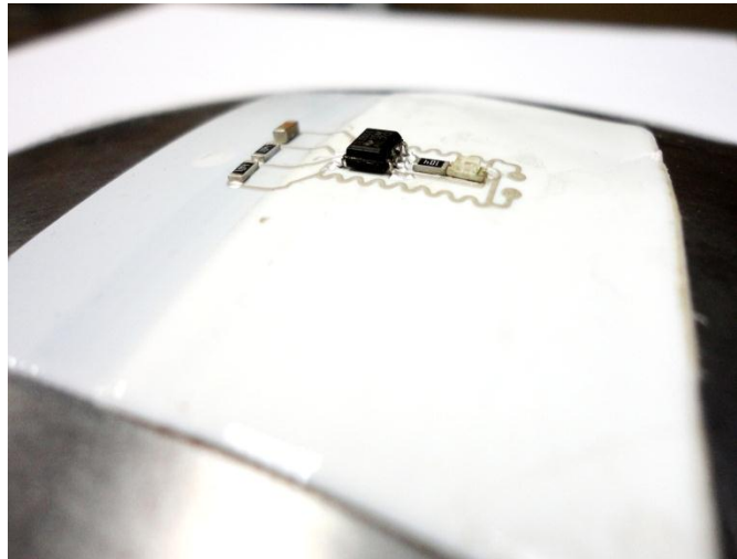
Figure 14 - Completed test circuits built with DPAM process. The left photo is on a flat surface, the right photo is a curved surface.
