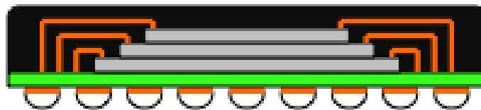
Figure 1. Progressively tiered die-stack and wire-bond package assembly.
