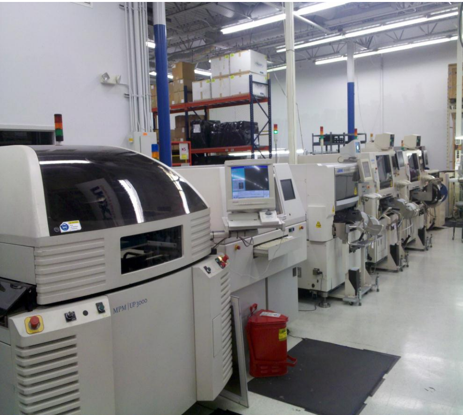
MPM UltraPrint 3000 – Screen Printing 5mil Laser Etched Solder Stencil
