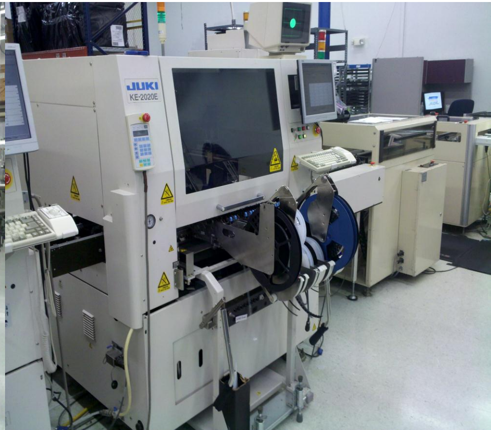
Juki KE-2020E SMT Placement Platform +/- 30 micron accuracy
