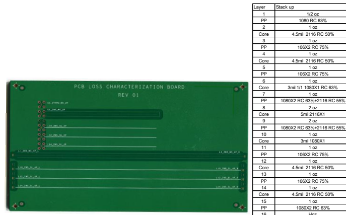
Figure 15 – Test pattern and stackup design of low loss material A
