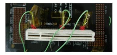
Thermocouples attached at various locations to measure thermal profile
