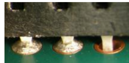
Copper dissolution and insufficient hole fill. Ref: Celestica 2007
