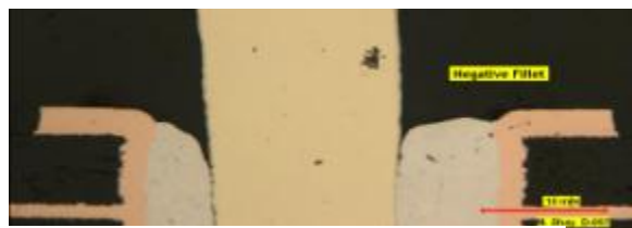
Figure 19: Negative Fillet from Wave Soldering
