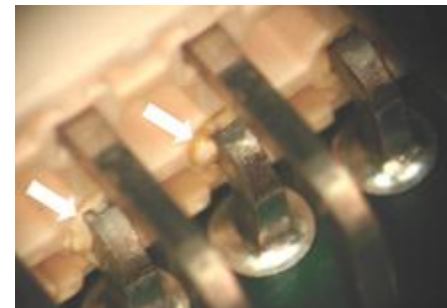
Plastic connector housing deformation from PTH rework heat. Ref: IBM 2007
