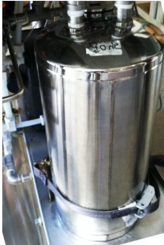
Photo 2 Stainless absorptive media tank (1/2 ft 3 shown)
