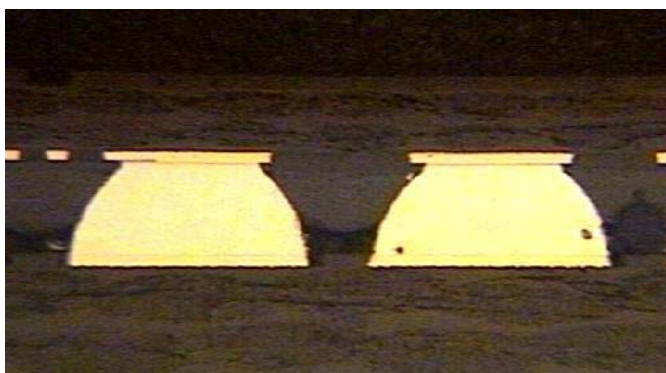
Figure 13 - BGA 196/NC-7 Pb-Free Paste The joint exhibits excellent wetting to the PCB pad and minimal voiding.
