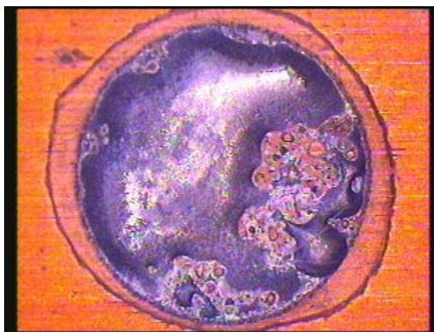
Figure 3 - OA-6 Example of Poor Wetting on OSP Coupon - Non-Wet and De-Wet Conditions Associated with this Paste.
