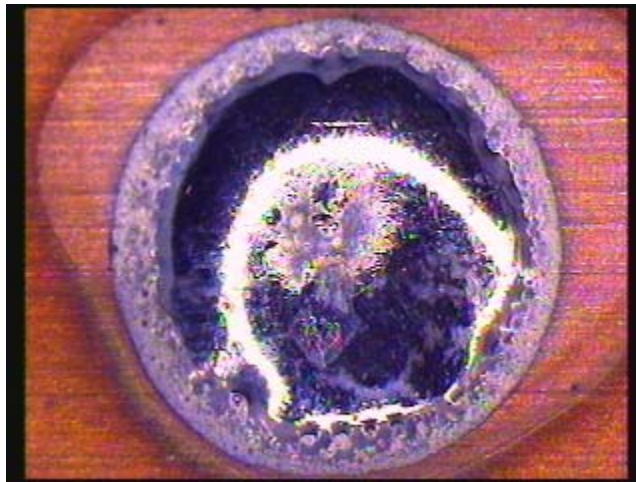
Figure 5 - OA-4 Example of Good Wetting on OSP Coupon –
