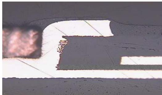
**Figure 3 – Cross-section of Board Using 24 µm Capacitance Layer with Micro-Via**
