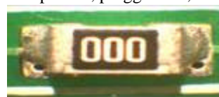
Figure 6 - Via in pad examples with Silver plated board finish
