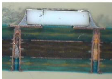
Figure 3 - Cross sections showing examples of .008" finished hole diameter plugged vias with various component packages and board finishes
