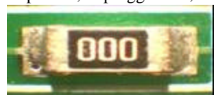
Figure 6 - Via in pad examples with Silver plated board finish
