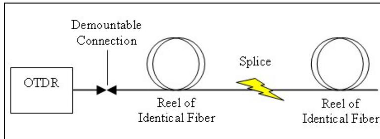
**Figure 4 - Schematic diagram of OTDR Test Setup for Splice Loss Measurement**
