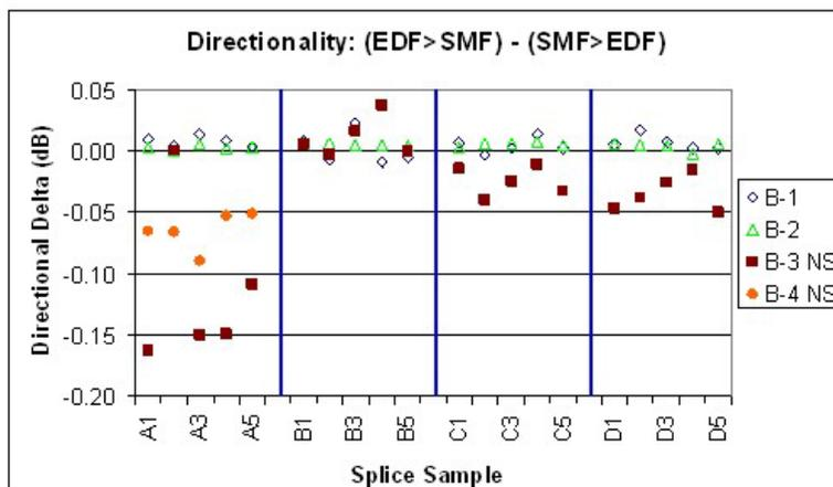
**Figure 9 - Round-Robin Directional Data for SMF-EDF Splices, at 1310 nm (Using BFA Methods of Appendix C) - A-D are Fiber Combinations and B-1 to B-4 are User Test Setups (See Table 1).**
