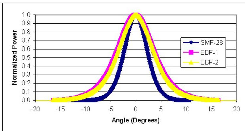
Figure 11 - Normalized Power Over  $\pm 20^\circ$  (Linear Scale)
