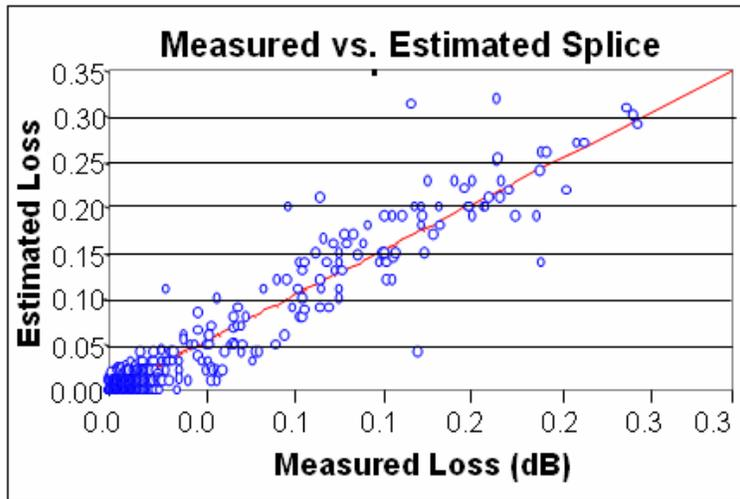
**Figure 1 - Correlation of the Splicer Estimator and Measured Loss (Typical Values Shown)**
