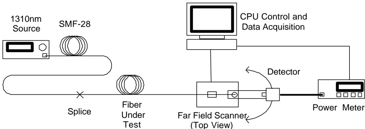
The  $1/e^2$  points of the intensity distribution give the numerical aperture (NA) of the fiber. The mode field diameter (MFD) is  $\mu 1/NA$ .
