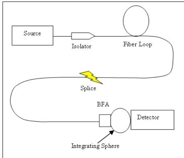
**Figure 2 - In-Line Method for Similar Fibers**
