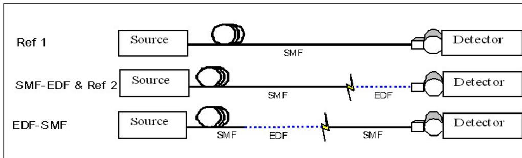
**Figure 3 - BFA Method Setup for Measuring Dissimilar Fibers in Two Directions**
