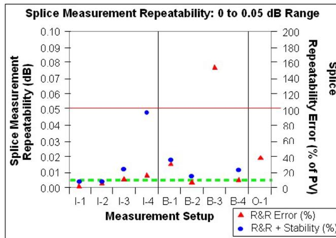
**Figure 7 - Splice Measurement Repeatability over the Low Loss Range for All Test Methods for Similar Fiber Splices**
