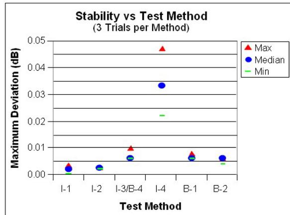
**Figure 6 - Stability of the different test methods**
