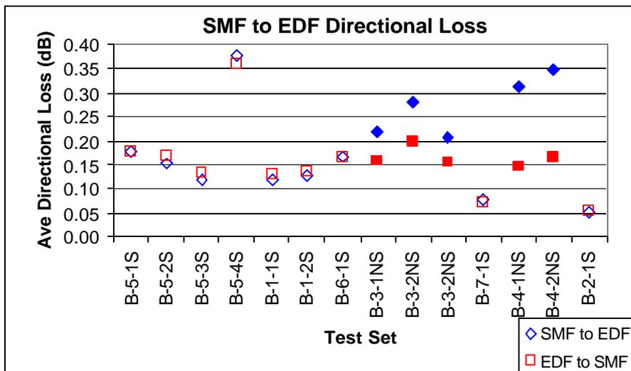
Loss data for SMF-EDF splices, measured in each direction at 1310 nm (using BFA methods 1 & 2 ). Set-ups B-3 and B-4 without an integrating sphere (NS) are shown as solid symbols.
