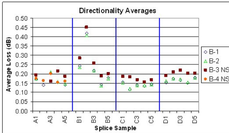
Figure 10 - Round-Robin for SMF-EDF Splices, Values for Each Direction are Combined and Averaged
