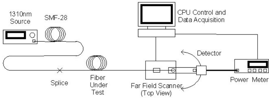
**Figure 5 - Schematic of the Far Field Scanning System**
