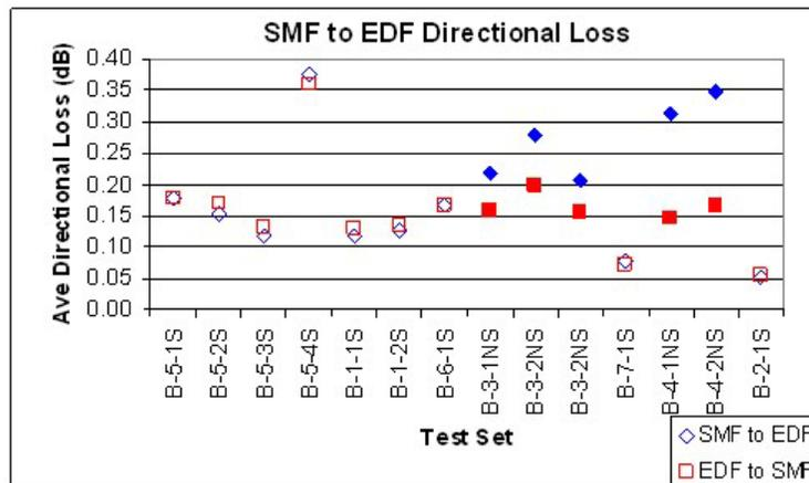
**Figure 8 - Loss Data for SMF-EDF Splices, Measured in Each Direction at 1310 nm (Using BFA Methods of Figure 3 and Appendix C). Set-Ups B-3 and B-4 without an Integrating Sphere (NS) are Shown as Solid Symbols**
