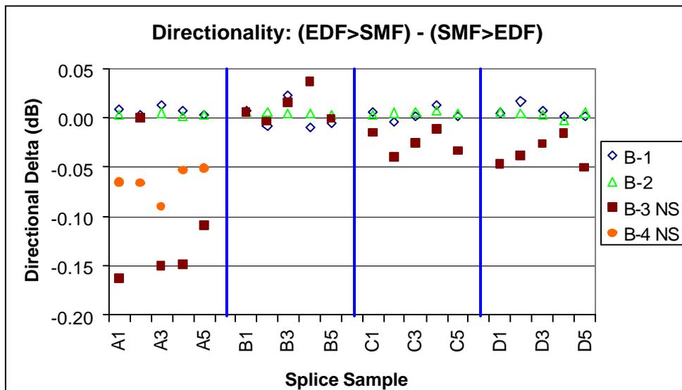
Round-robin directional data for SMF-EDF splices at 1310 nm (using BFA site-to-site method). A to D are fiber combinations and B-1 to B-4 are user test setups. The largest in directionality is found for user set-ups B-3 & B-4, both without an integrating sphere.
