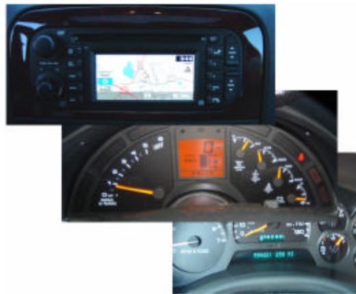
Figure 2 - Automotive Digital Displays using a Range of Technologies
