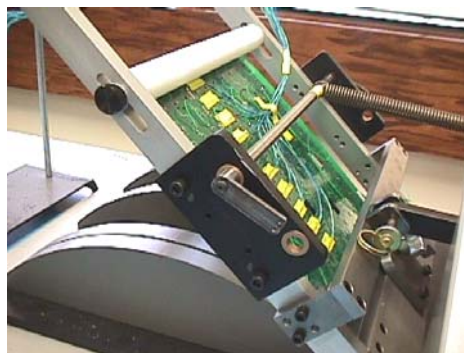
Figure 2 - Board-Bending Apparatus with 200mm Radius of Curvature Operates at 1 Hz. 100 Daisy Chain Parts are Tested Simultaneously - 10 Parts per Row Constitute a Population with a Given Imposed Strain Energy State - Wires seen coming off the Board are attached to Strain Gages associated with each Row Position
