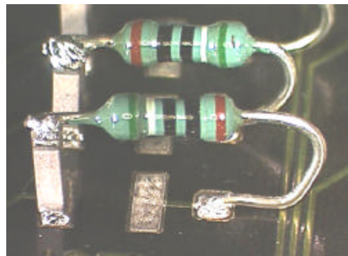
Figure 16 - Modification N - 1808 Capacitor "Billboarded"/Axial Resistor
