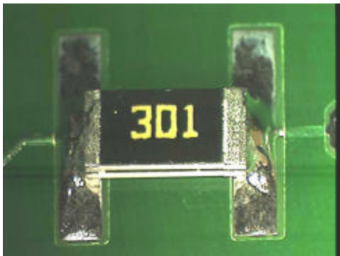
Figure 5 – Modification C – Two 2010 Resistors “Piggybacked”
