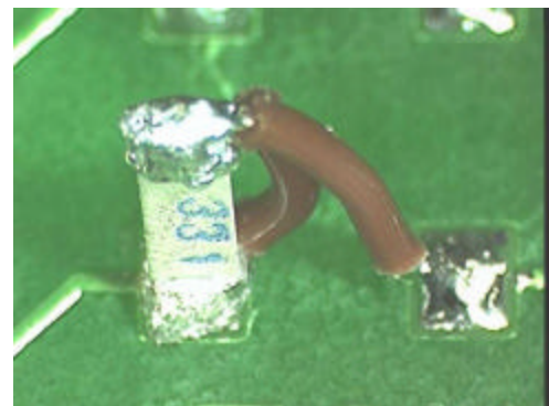
Figure 10 - Modification H - 1805 Capacitor “Tombstoned” With 2 Add Wires
