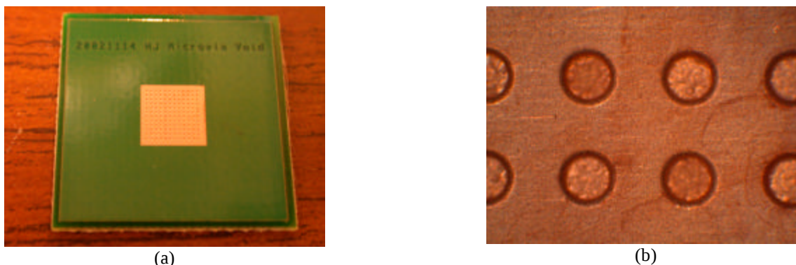
Figure 1 - Microvia Test Boards Used for Studying Effect of Solder Alloy Composition on Voiding, (a) Overall View of Test Coupon, (b) Closed Up Look of Test Coupon
