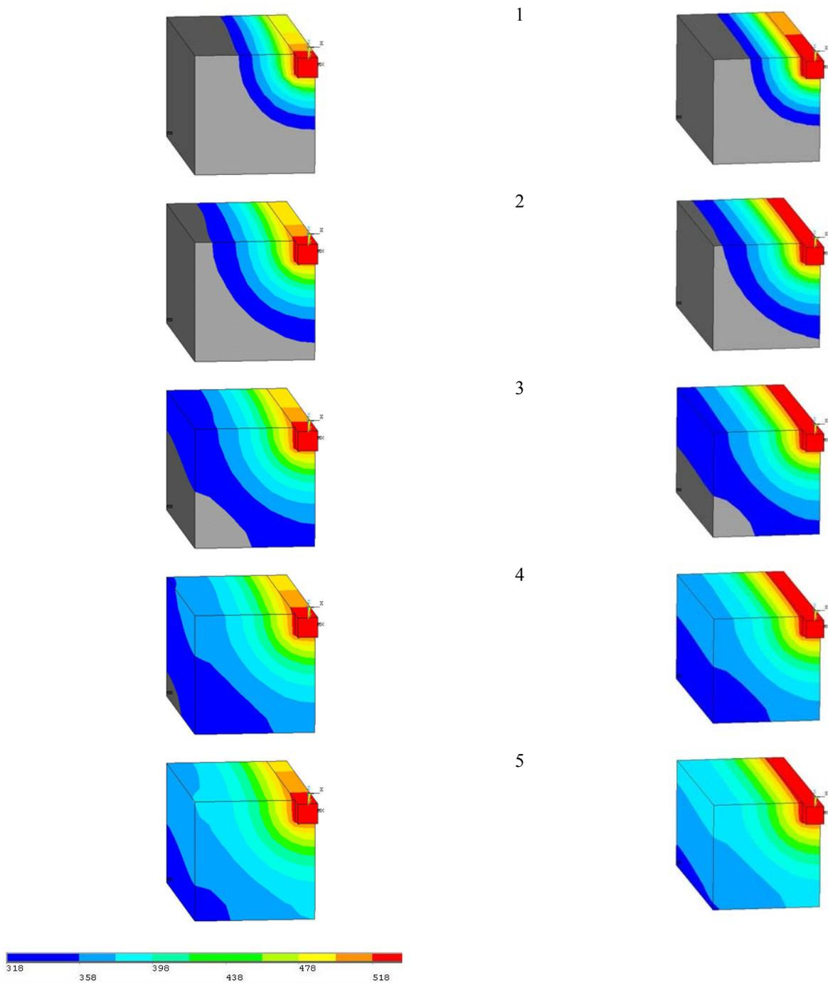
**Figure 10 - Thermal Results Of Simulated Overmolded, Phosphor Bronze (Left) and Copper Iron (Right) Contacts, Exposed to Lead Free Wave Solder Conditions for 5 Seconds, Incorporating Phase Change Effects**
