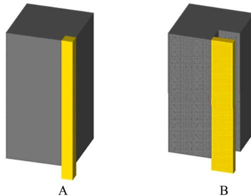
**Figure 1 - Quad Symmetric Geometry Used for FEM Analysis of Contacts Inserted in a Plastic Body. A) Overmolded Contact with Plastic to Metal Interfaces on Four Sides and B) Staked Contact with Plastic to Metal Interfaces on Parts of Two Sides**
