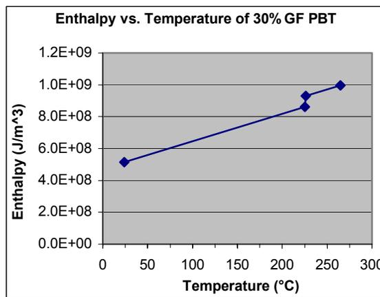
Figure 13 - Enthalpy vs. Temperature for 30% Glass-Filled PBT
