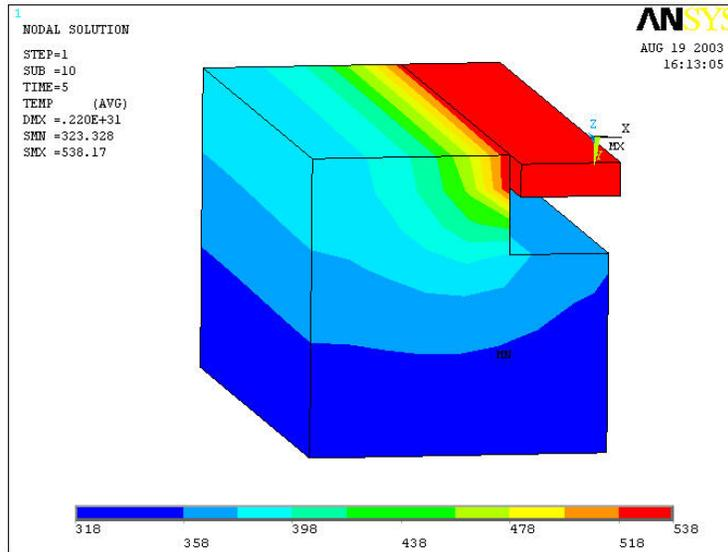
**Figure 17 - Thermal Results of Simulated Staked, Copper Iron Contacts, Exposed to Lead Free Wave Solder Conditions for 5 Seconds, Incorporating Phase Change Effects**
