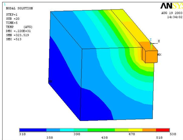
**Figure 2 - Thermal Results of Simulated Overmolded, Phosphor Bronze Contacts, Exposed to Sn/Pb Wave Solder Conditions for 5 Seconds**
