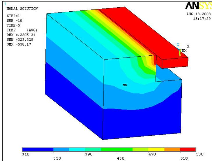
**Figure 9 - Thermal Results of Simulated Staked, Copper Iron Contacts, Exposed To Lead Free Wave Solder Conditions for 5 Seconds**
