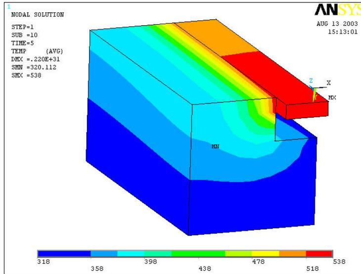
**Figure 8 - Thermal Results of Simulated Staked, Phosphor Bronze Contacts, Exposed to Lead Free Wave Solder Conditions for 5 Seconds**
