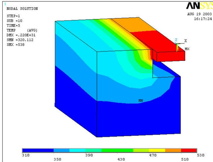
**Figure 16 - Thermal Results of Simulated Staked, Phosphor Bronze Contacts, Exposed to Lead Free Wave Solder Conditions for 5 Seconds, Incorporating Phase Change Effects**
