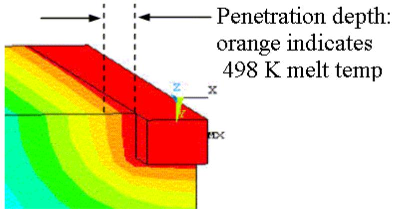
**Figure 18 - Maximum Melt Temperature Penetration Depth into Plastic**
