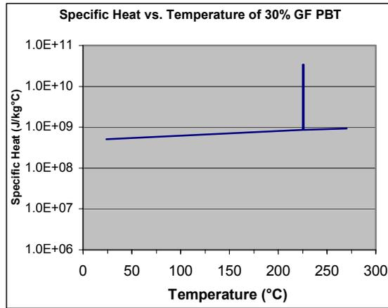
Figure 12 - Specific Heat vs. Temperature for 30% Glass-Filled PBT.
