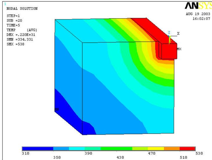
**Figure 15 - Thermal Results of Simulated Overmolded, Copper Iron Contacts, Exposed to Lead Free Wave Solder Conditions for 5 Seconds, Incorporating Phase Change Effects**
