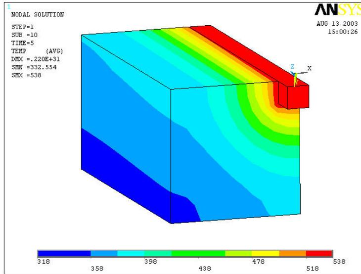
**Figure 7 - Thermal Results of Simulated Overmolded, Copper Iron Contacts, Exposed to Lead Free Wave Solder Conditions for 5 Seconds**
