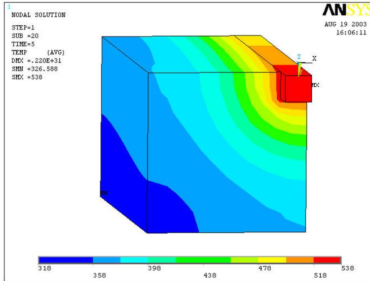
**Figure 14 - Thermal Results of Simulated Overmolded, Phosphor Bronze Contacts, Exposed to Lead Free Wave Solder Conditions for 5 Seconds, Incorporating Phase Change Effects**
