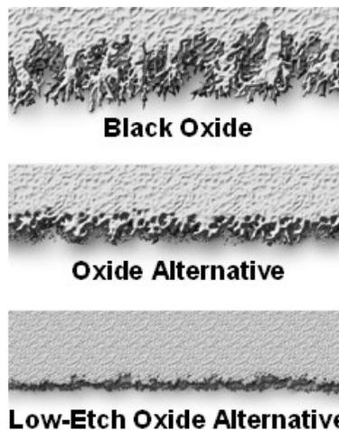
**Figure 3 - Schematic Representation of Oxide and Oxide Alternative Surfaces**
