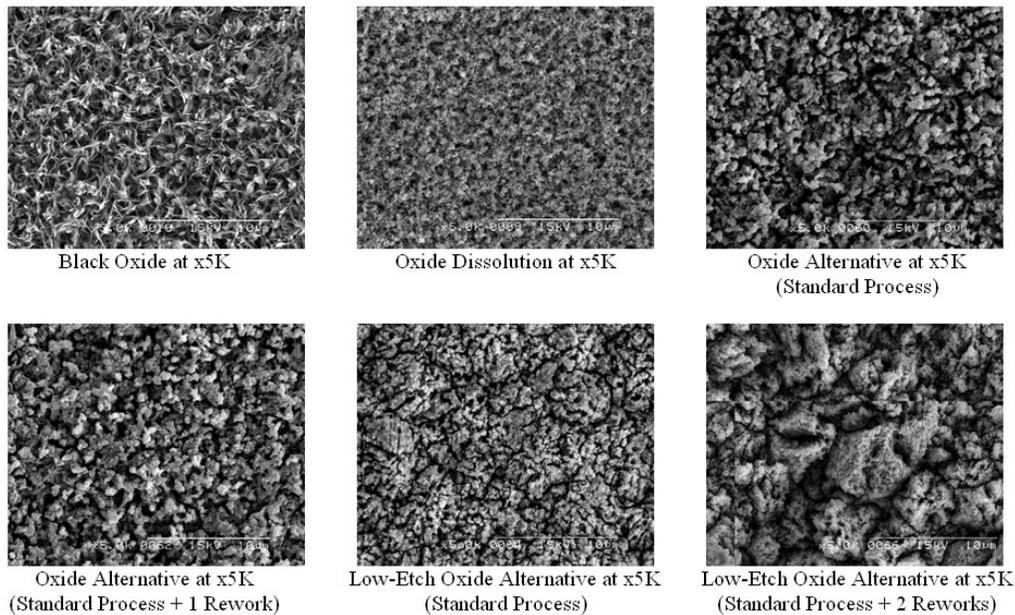
**Figure 8 - SEM Pictures of Process Factors**
