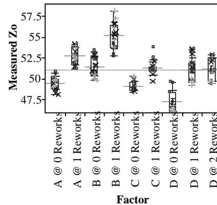
Figure 12 - Measured Impedance
