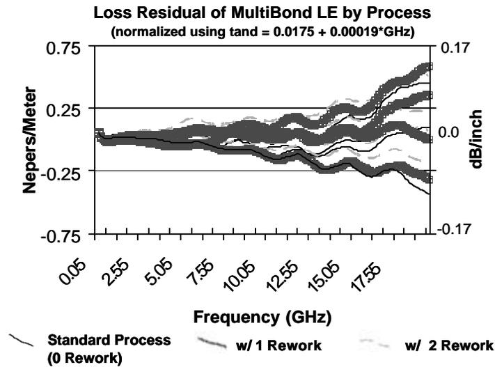
Figure 19:  $a_{\text{measured}} - a_{\text{modeled}}$  for Low-Etch Oxide Alternative
