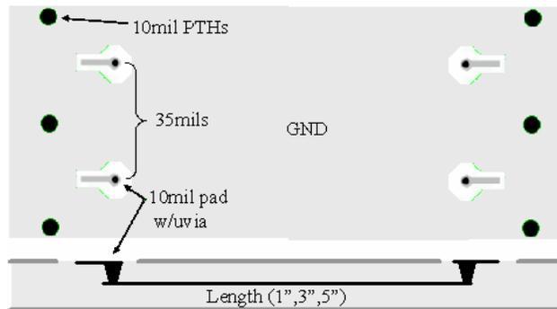
Figure 7 - Test Structure Schematic
