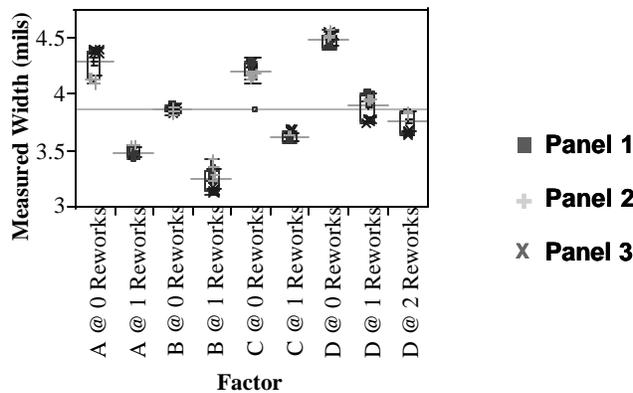
**Figure 9 - Measured Trace Widths**
