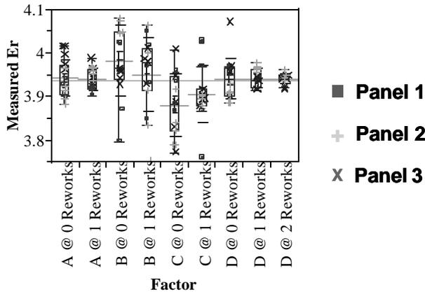
Figure 11 - Measured Dielectric Constant
