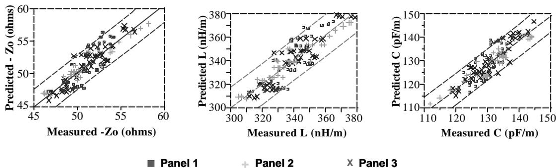
Figure 14 - Modeled vs Measured Transmission Properties.
