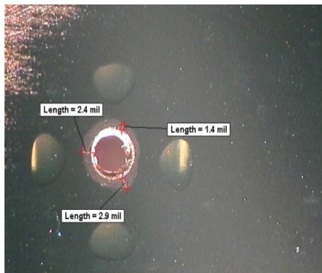
Figure 12A - Reduced Oxide Coupons Showing Pink Ring
