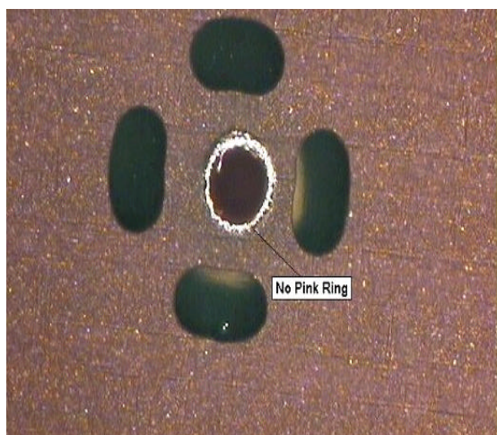
Figure 12B - Organo-metallic Process for MLB Coupons-no Pink Ring Found
