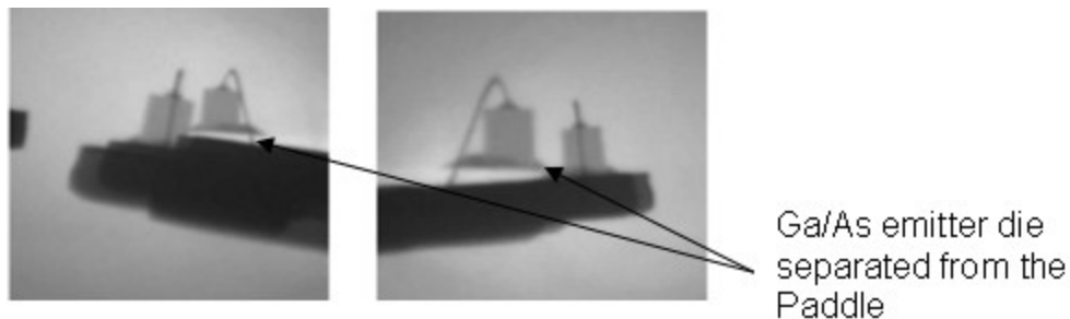
Figure 14 – Transmission X-ray Inspection Revealing die Delamination in Optocoupler B
