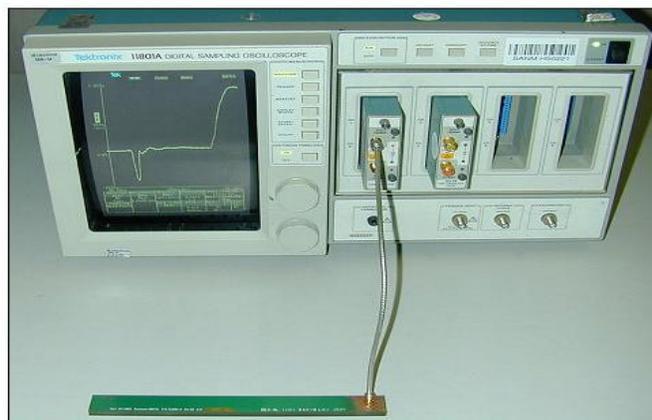
Figure 1 - Typical TDR Setup with a 6” Test Coupon
