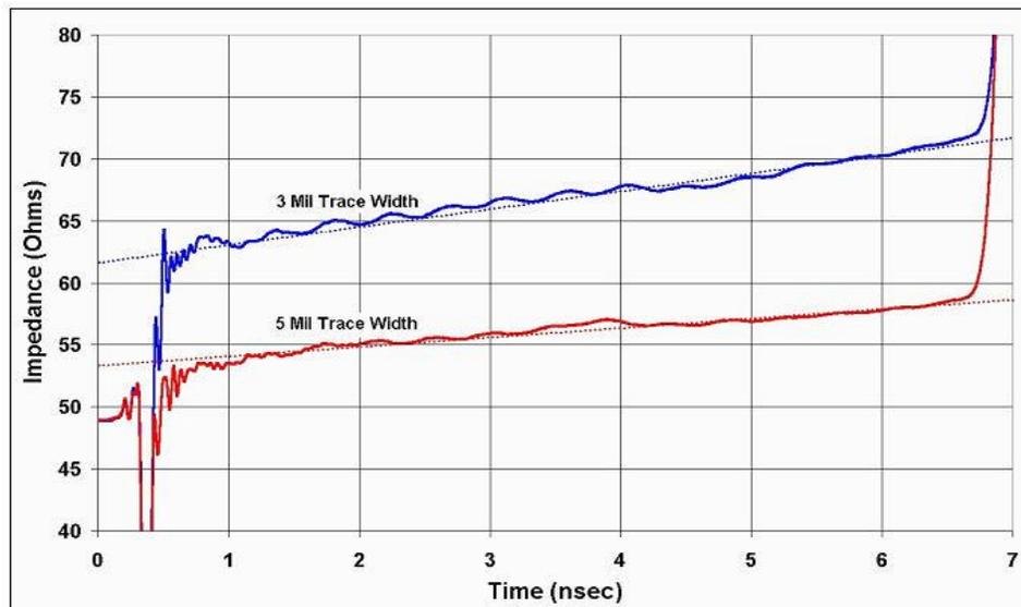
Figure 9 - TDR Measurements Made Comparing 3 and 5mil Trace Widths. Note the Higher Initial Impedance Due to Skin Effect Loss. The 3mil Trace Width also has a Higher Rate of Impedance Change
