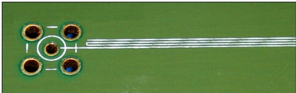
**Figure 7 - SMA Launch with 5mil Wide Trombone Traces and a 9mil Pitch**
