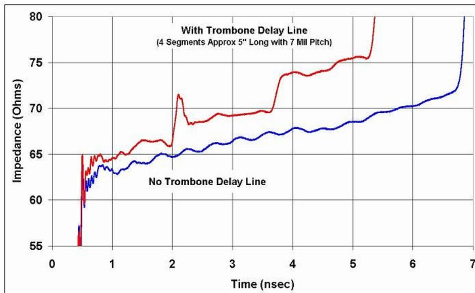
**Figure 8 - TDR Measurements Made Across Traces with Overlapping Segments (trombone type layout) Versus no Overlap (straight) Test Trace. Both Absolute and Periodic Impedance is Higher with the Trombone Designed Traces**
