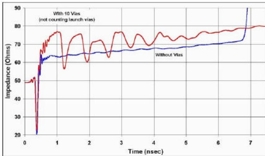
**Figure 12 - TDR Measurements Made Comparing Test Traces with 10 Vias in the Signal Path Versus no Vias in the Signal Path. An Obvious Improvement in Trace Impedance Characterization is Seen with no the Removal of Vias in the Signal Path**
