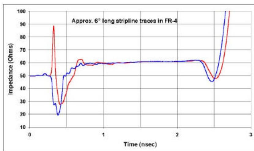
Figure 6 - TDR Response from a Polar Probe (in red) and Single Coaxial Cable (blue). Removing the Top Layer of Solder Mast Allows the Use of the Top Plane (GND) as a Return Signal Path thus Reducing overall Inductance
