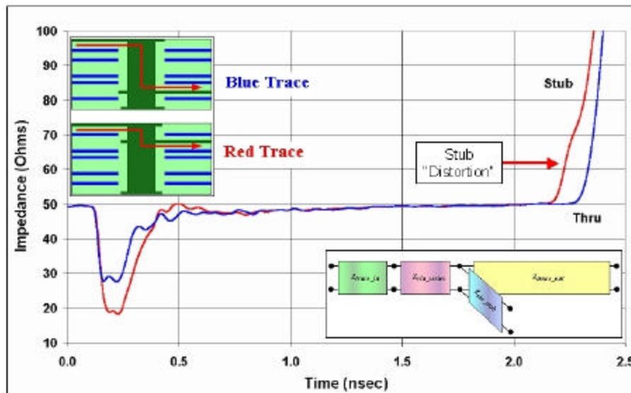
**Figure 13 - Two TDR Responses from a 6-inch Long 50-ohm Stripline on Layers 2, and 18 in a 21 Layer Test Coupon, Made Using FR-4 Material**
