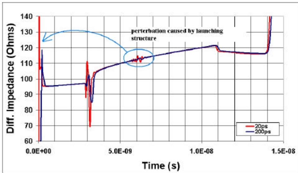
**Figure 11 - Two TDR Responses from a 20 and 200ps RT Step Signal. Note the Differences in the Features of the Launch Via and the Discontinuity is the Middle of the Trace Caused by Back Reflections Between the Launch Via and the Connector. For the RT of 200ps, the Anomaly is not Present**
