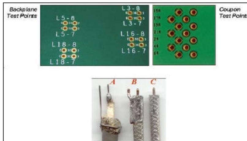
**Figure 3 - Test Coupon and Backplane Test Points with Homemade Probes used to Test Traces. Probe A Carries More Inductance Than Probe C, and Therefore is Not as a Favorable for Impedance and Propagation Measurements**
