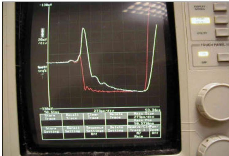
Figure 4 - TDR Using Probe Type A (white) as Compared to Probe Type B (red) Note the Inductive Effects of the Ground (Return Current) Pin have of the TDR
