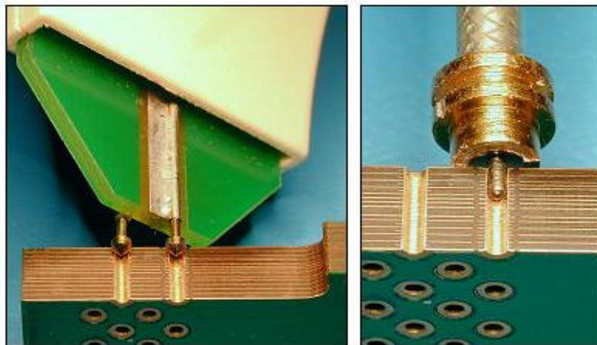
Figure 5 - Test Probes in Coupon (left) – Polar Probe, Useful at about 50ps RT. Single Coaxial Cable (right). Removing the Top Layer of Solder Mast Allows the Use of the Top Plane (Ground Layer) as a Return Signal Path thus Reducing Overall Inductance
