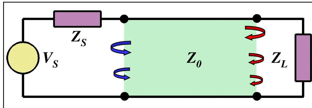
$$\Gamma_{\text{Load}} = \frac{Z_L - Z_0}{Z_L + Z_0}$$
