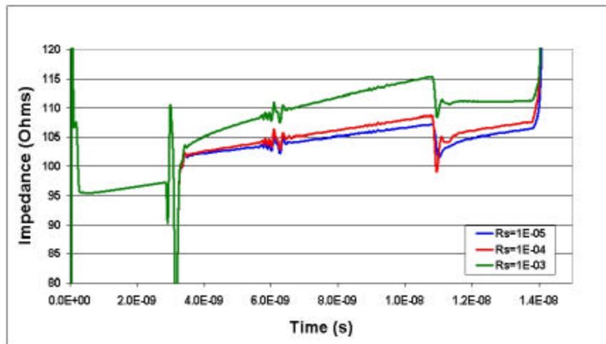
Figure 10 - Three Different Levels of Skin Effect Loss Showing the Contribution to Impedance Changes.  $R_s$  Measured in Units of  $W/m * \sqrt{Hz}$
