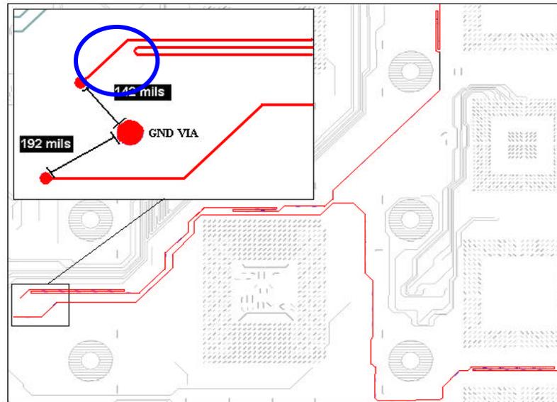
**Figure 2 - PCB Outline with Test Traces in Blue, Showing Different Signal / Gnd Pitch, Folded "Trombone" Traces and Close Proximity to Other Packages**
