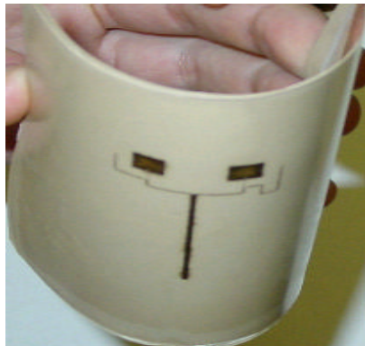
Figure 11 - Double-sided Flex Antenna from 425 Micron Core Laminate Illustrating the Flexible Nature of the Dielectric 11
