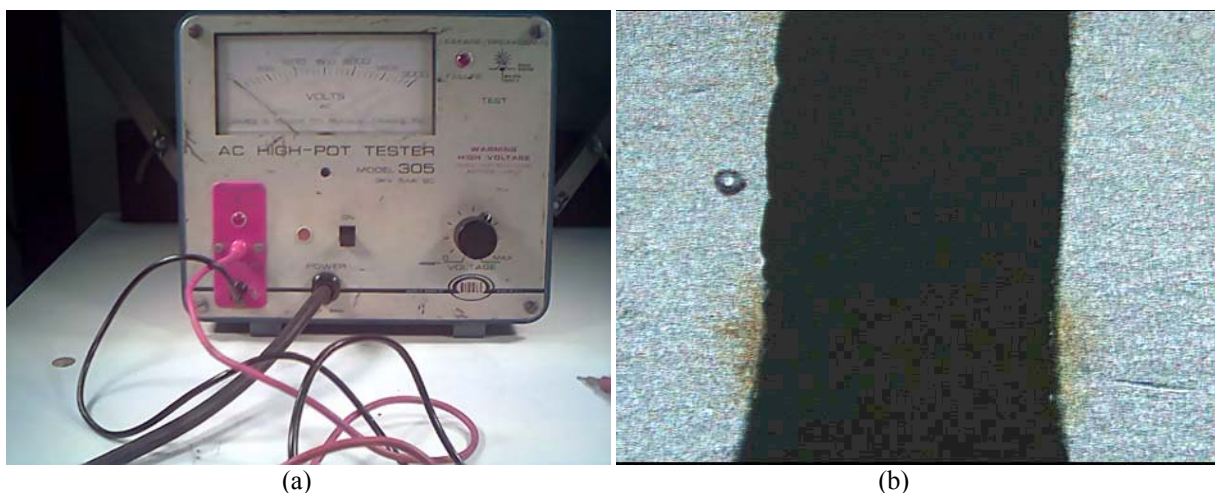
Figures 2ab - High-Voltage Source Used in Withstand Voltage Test; Test Pattern after Electric Arc
