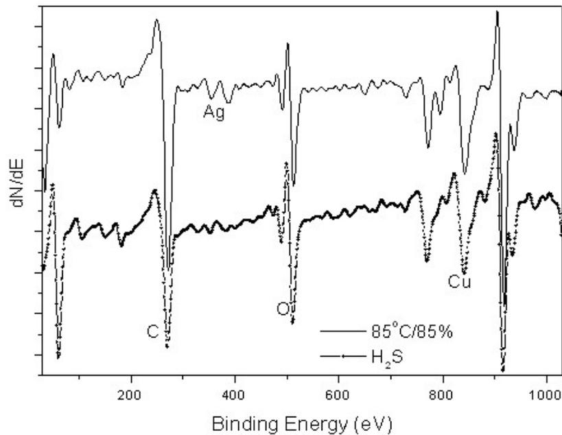
**Figure 5 - Auger Surface Analysis of 3.4  $\mu\text{m}$  Silver from PROCESS A after the Humidity Test (top), and 13  $\mu\text{m}$  Silver from Process A after Hydrogen Sulfide Test (bottom)**
