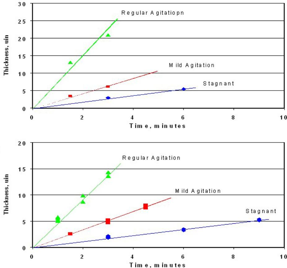
Figure 1 - Silver Thickness for Process A (top), and for Process B (bottom)
