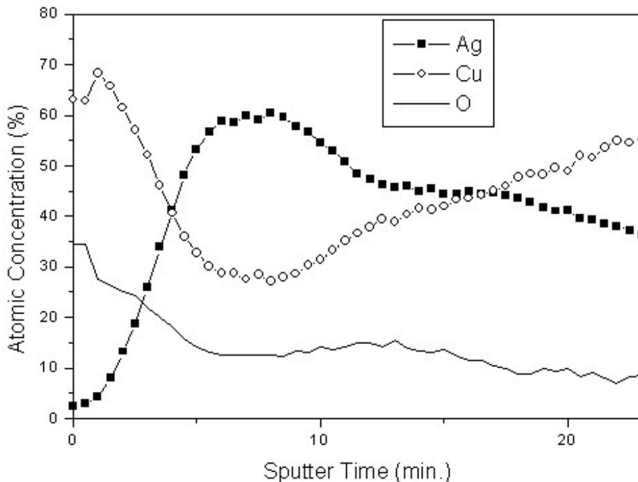
**Figure 6 - Auger Depth Profile of the 3.4  $\mu\text{m}$  Silver from Process A after 24-Hour Exposure to Humidity Test**
