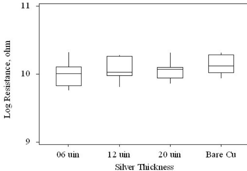
**Figure 9 - Box-Whisker Plot of Electro-Migration Resistance for Silver Plated from Process B (Measured after 500 Hour Exposure to 85°C/85%RH under a 10-V bias)**
