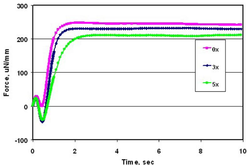
**Figure 7 - Effect of Reflow on Wetting Balance Curve of Silver Plated from Process B (6.5  $\mu\text{in}$  at Mild Agitation for 3 Minutes)**
