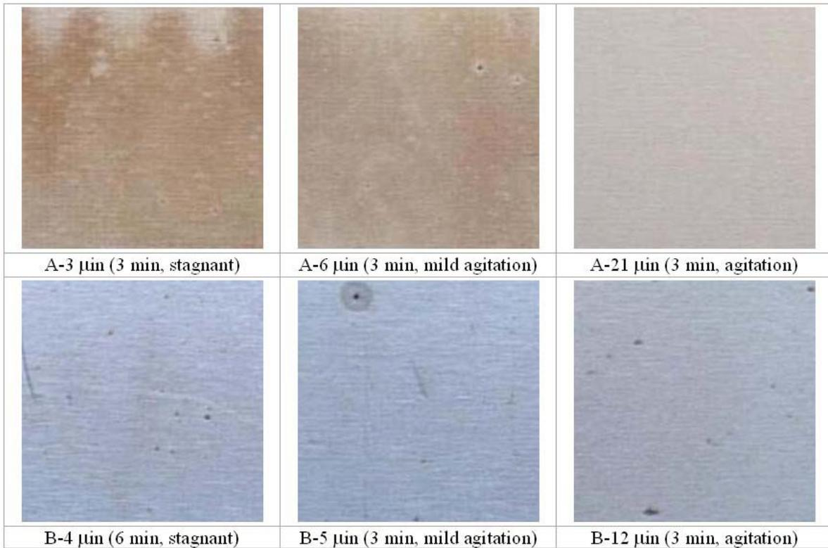
**Figure 3 - Appearance of Samples after 24 Hour Exposure to the Humidity Test for Silver Coated from Process A (top) and Process B (bottom)**
