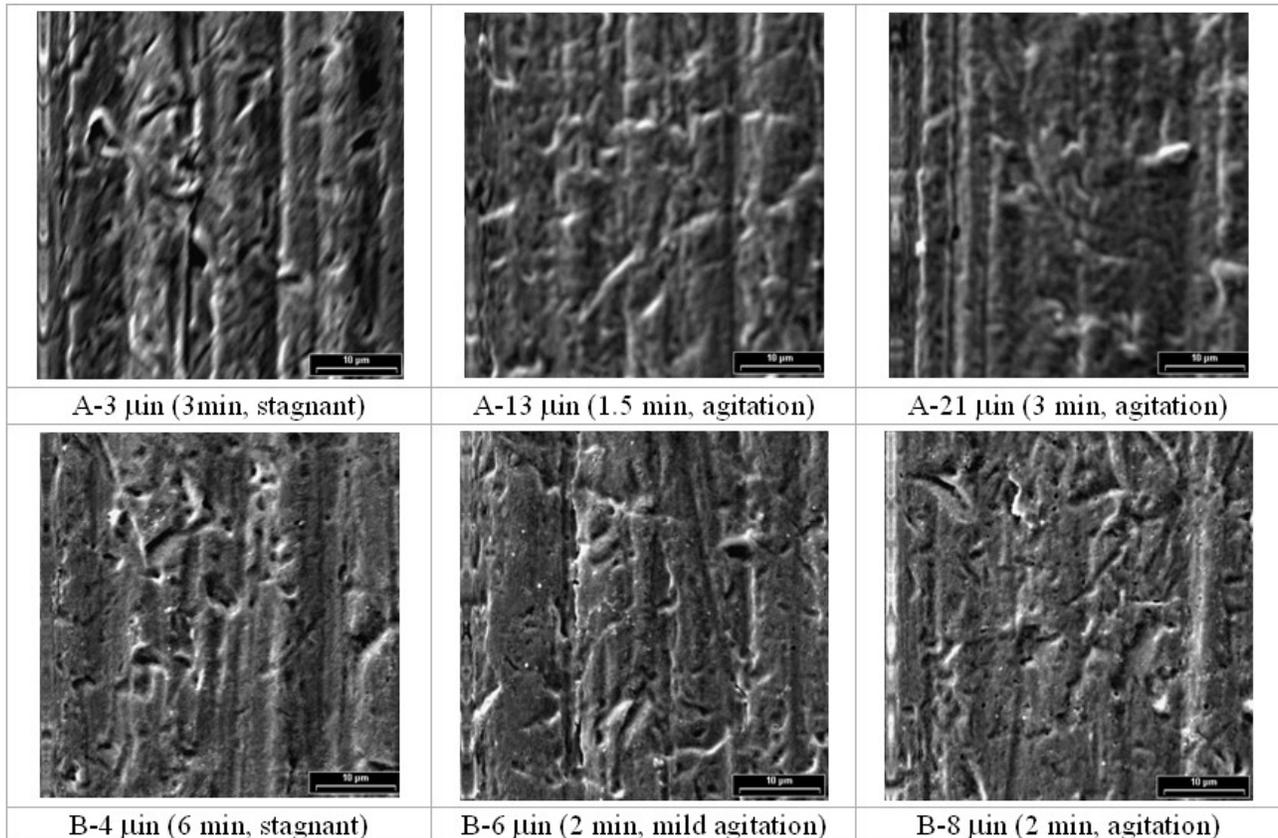
**Figure 2 - SEM Photomicrographs of Silver Coated from Process A (top) and Process B (bottom)**
