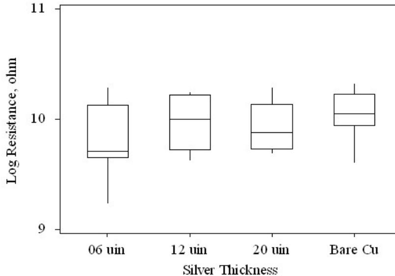
**Figure 8 - Box-Whisker Plot of SIR for Silver Plated from Process B (Measured after 96 Hour Exposure to 85°C/85%RH)**
