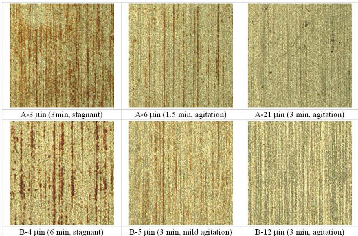
**Figure 4 - Appearance of Samples after 2 Minute Exposure to the Hydrogen Sulfide Test for Silver Coated from Process A (top) and Process B (bottom)**
