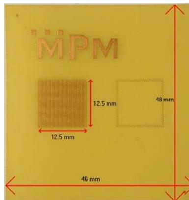
**Figure 1 - High Density Substrate – Test Vehicle**
