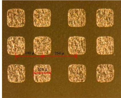
**Figure 2: High Density Substrate - UBM**
