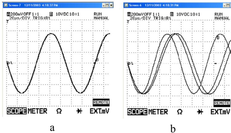
**Figure 8(a) - Waveform of 9.2 KHz and 8(b): Waveform of 9.2 KHz with FM**
