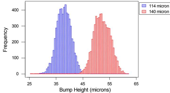
**Figure 7 - Bump Height Distribution for 114 and 140 micron Square Opening**
