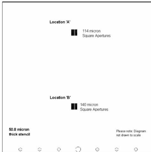
**Figure 3 - Stencil Design for HDS**
