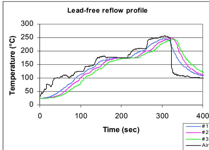
**Figure 5 - Lead-Free Reflow Profile**
