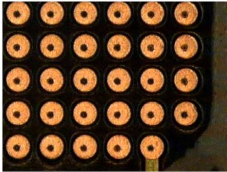
**Figure 6 - An example of the PCB Layout for 0.4 mm Pitch CSP (Microvia In Pad)**
