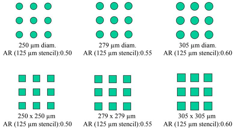
**Figure 4 – Stencil Aperture Shapes, Sizes and Area Ratios Studied for 0.4 mm Pitch CSP Components**
