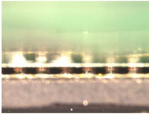
**Figure 8 – Example of Open Solder Joint with “Window” PCB Pad Design - The Open Joint is Third from the Left**
