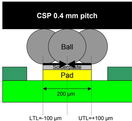
**Figure 11 – Tolerance Limits for 0.4 mm Pitch CSP and  $200 \mu\text{m}$  PCB Pad Size**
