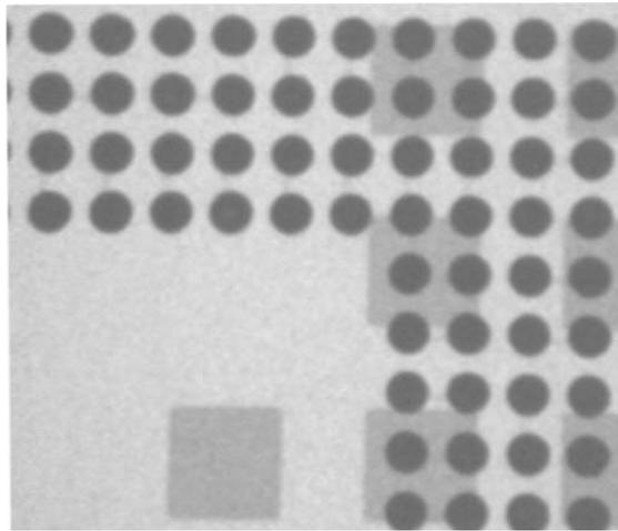
**Figure 10 - 0.4 mm Pitch CSP, Misaligned ~50% in Pick & Place Process, after Reflow, Using CSP with Sn/Ag/Cu Balls and Sn/Ag/Cu Paste**
