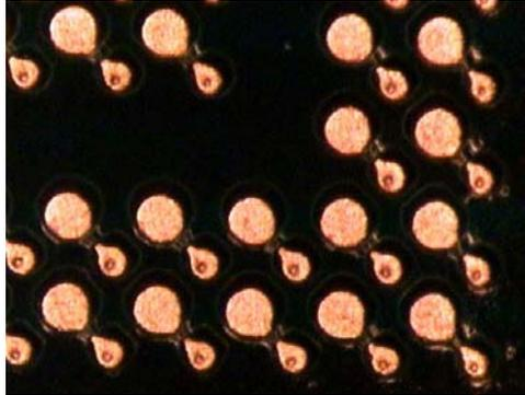
**Figure 7 – An Example of the PCB Layout for 0.5 mm Pitch CSP (No Via In Pad)**
