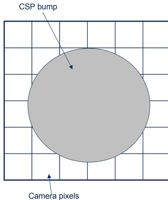
**Figure 12 – A schematic Illustration of the Camera Pixels versus the Bump Size**
