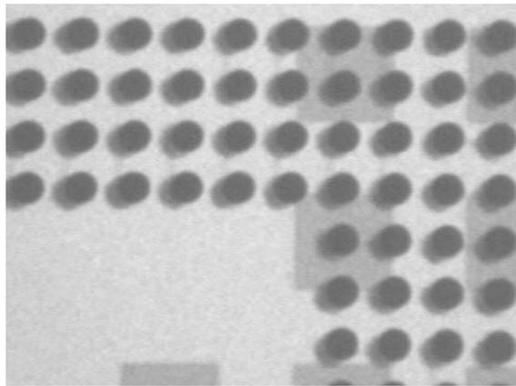
**Figure 9 - 0.4 mm Pitch CSP Misaligned ~50% in Pick and Place Process Using CSP with Sn/Ag/Cu Balls and Sn/Ag/Cu Paste**
