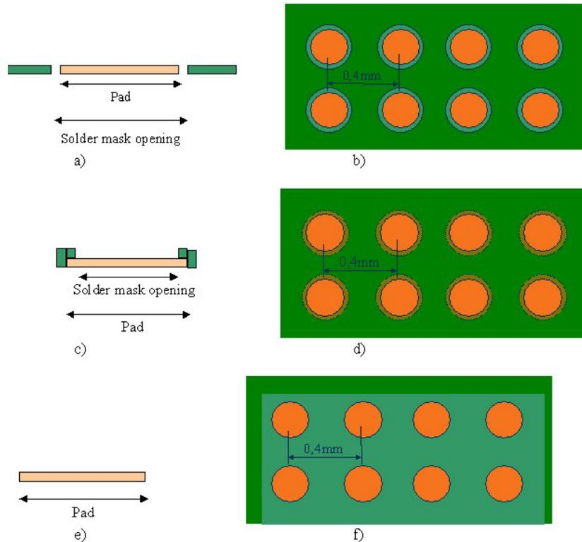
**Figure 3 – Schematic Illustrations of the Three Different Pad Designs Studied, a) NSMD, Side View, b) NSMD, Top View, c) SMD, Side View, d) SMD, Top View, e) “Window,” Side View, f) “Window,” Top View**
