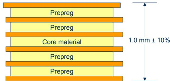
**Figure 2 – A Schematic Illustration of the Build-up Layers of the PCB**
