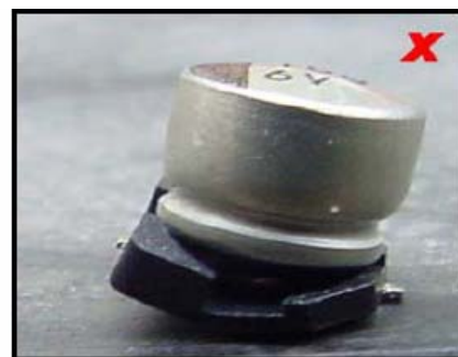
Figure 6c – Internal Component "Meltdown"
