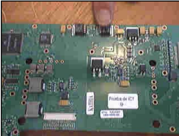
Initial Lead Free Reflow Solder Test: LF Solder paste: SnAg3.8Cu0.7
