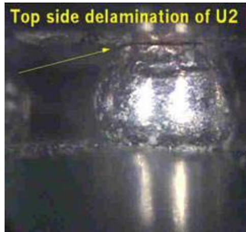
Delamination difficult to detect with x-ray
