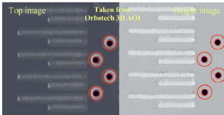
Figure 7 – Detecting Elements of the Same Height as the Covered pads (in this case, vias) Helps in Setting the Reference for Paste Measurement
