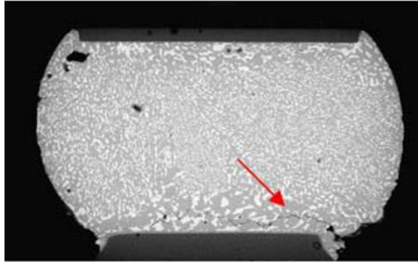
**Figure 9 – Fatigued Corner Joint**
