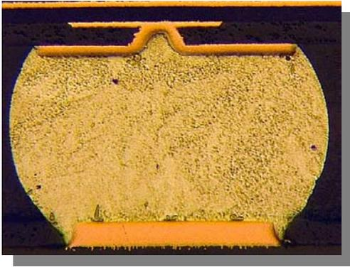
**Figure 6a - Representative Solder Joint**
