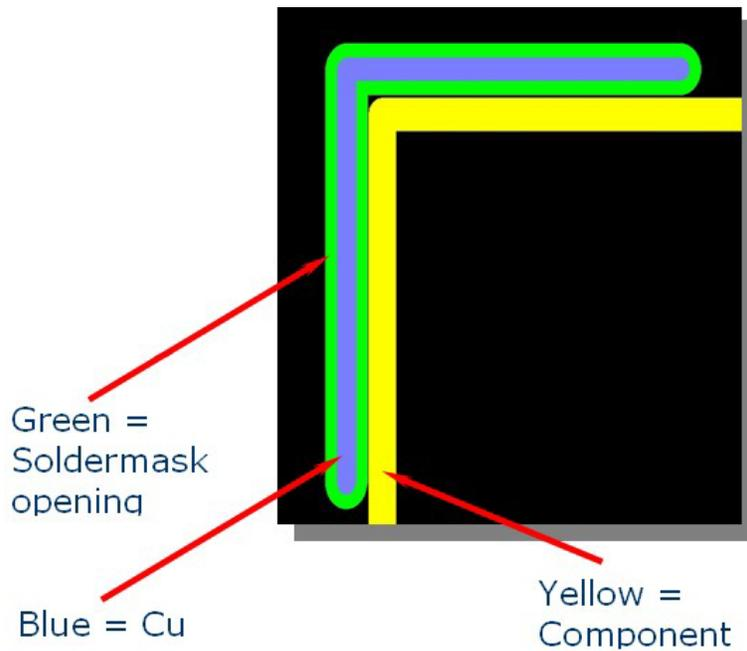
**Figure 14 - Solder Mask Registration Mark**
