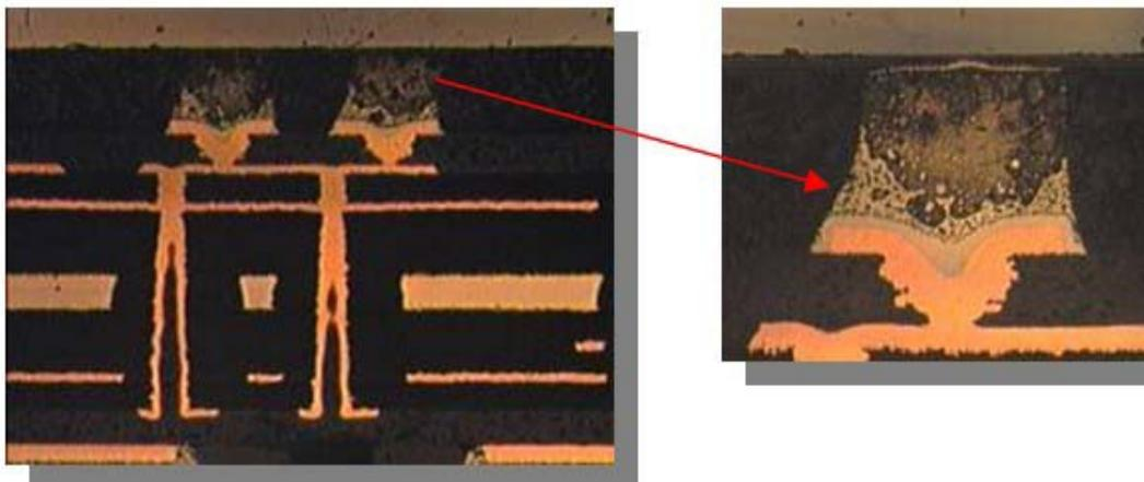
Figure 2 - Cross-Section of the 2577 I/O BGA High-Pb Flip Chip Bump Using Sn63/Pb37 Solder attach to PTFE Via-In-Pad
