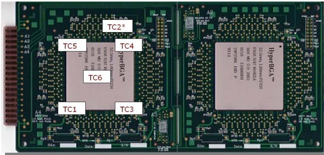
**Figure 5 - Thermocouple Locations – 5 Locations @ 2577 I/O device**
