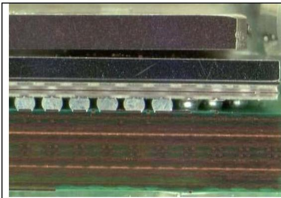
**Figure 7a - Flux-Only Rework Cross-Section Overview**
