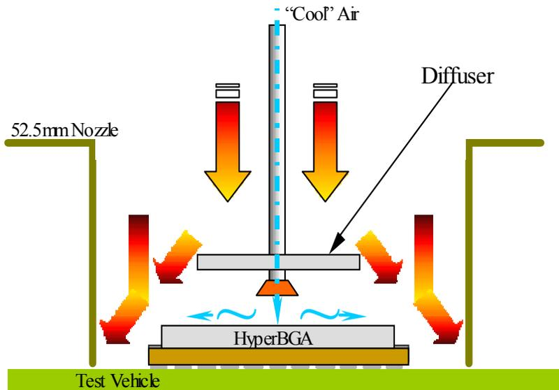
**Figure 15 - Rework Reflow Schematic Including Diffuser**
