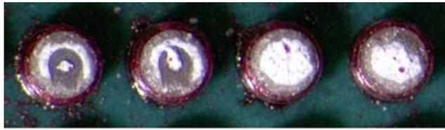
**Figure 12 – Dye Penetrant Testing of Centrally Located Solder Joints**
