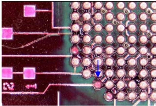
**Figure 10 – Dye Penetrant Testing of Corner Solder Joints**
