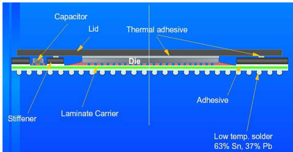
Figure 1 - 2577 I/O BGA Pictorial Cross-Section (IBM Packaging ASIC Overview (April 2001)).
