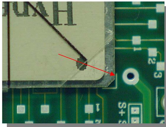
**Figure 13 - Cu Alignment Mark**
