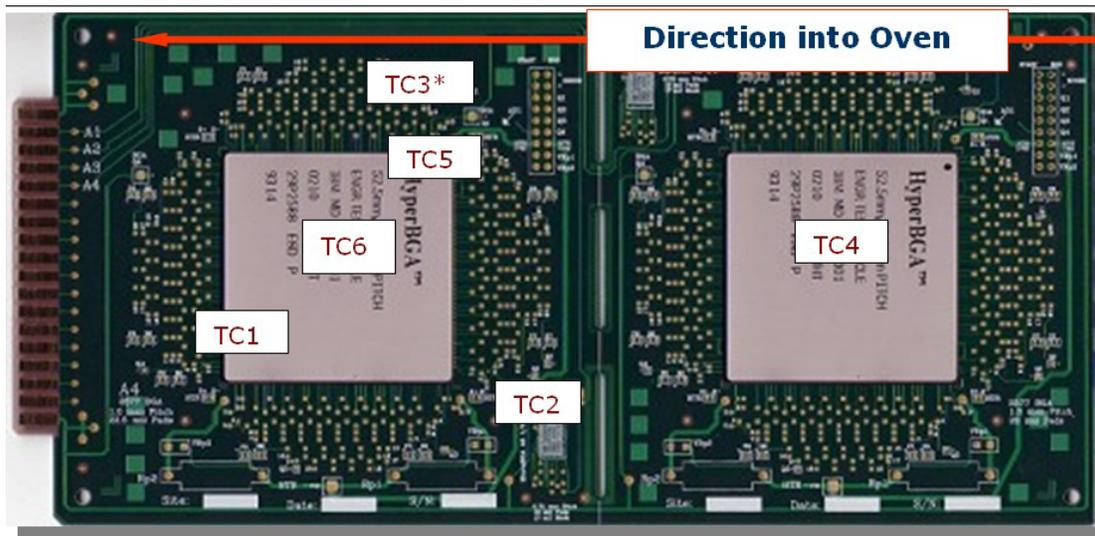
**Figure 6 - Thermocouple Locations – Across the Test Vehicle**
