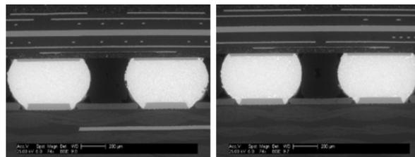
**Figure 11 – Solder Joints without Fatigue Cracks**
