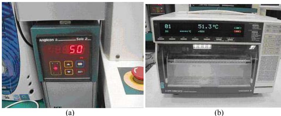
Figure 9 -The Chamber Temperature Read from (a) Heating Controller and (b) Thermocouple Recorder
