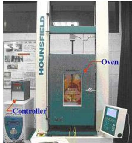
Figure 5 - The Micro-Force Material Testing Machine
