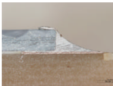
Figure 2 – Optical Image of 1206 Surface Mount Capacitor with a Hand Soldered SnPb Joint
