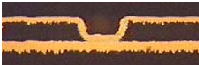
Figure 8 - Via Hole on Board Consisting of 10 \mu m Glass Fabric by UV-YAG Laser Drilling
