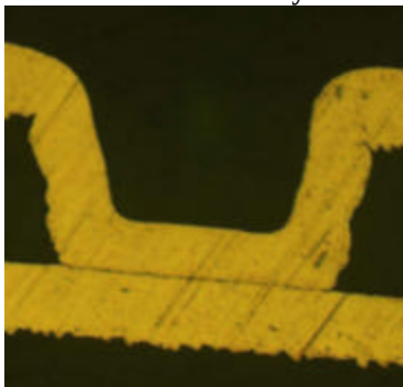
Figure 3 - Poor Desmear Before PTH
