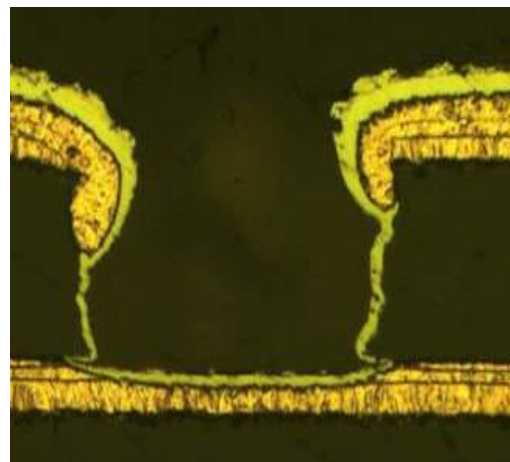
Figure 10 - Covered By Immersion Au/Ni
