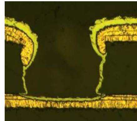
Large area of void in PTH
