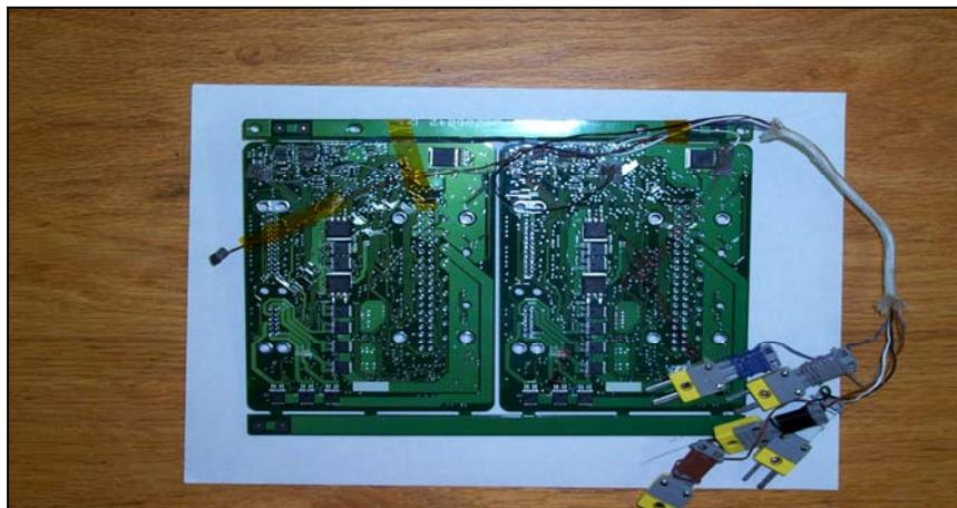
Figure 3 - Tested Product with Thermal Couples Attached
