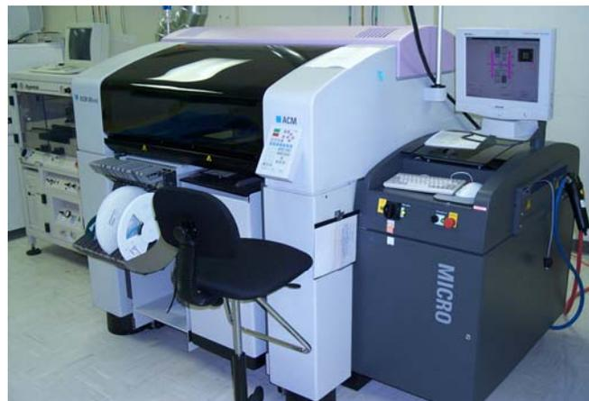
**Figure 9 - Assemble on ACM Placement**
