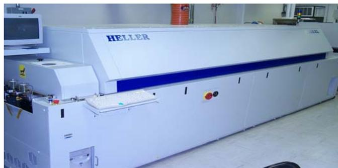
**Figure 10 - Heller Reflow Oven**
