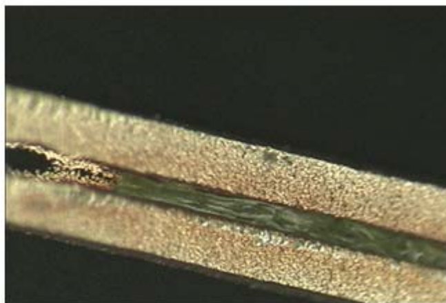
Figure 8 - Lack of Dry Film Stripping
