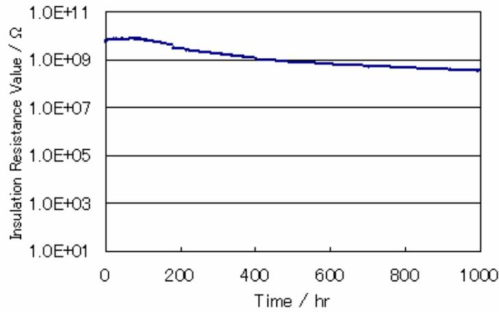
**Figure 7 - Insulation Reliability under the THB (85°C, 85%, 50V) Conditions**
