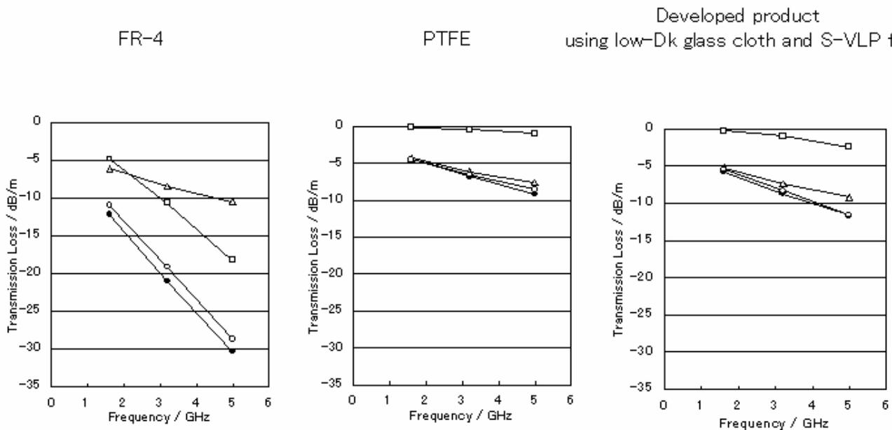
**Figure 12 - The calculated transmission loss value - Circle is Transmission loss, square is dielectric loss and triangle is conductive loss - Closed circle is measured value of transmission loss**
