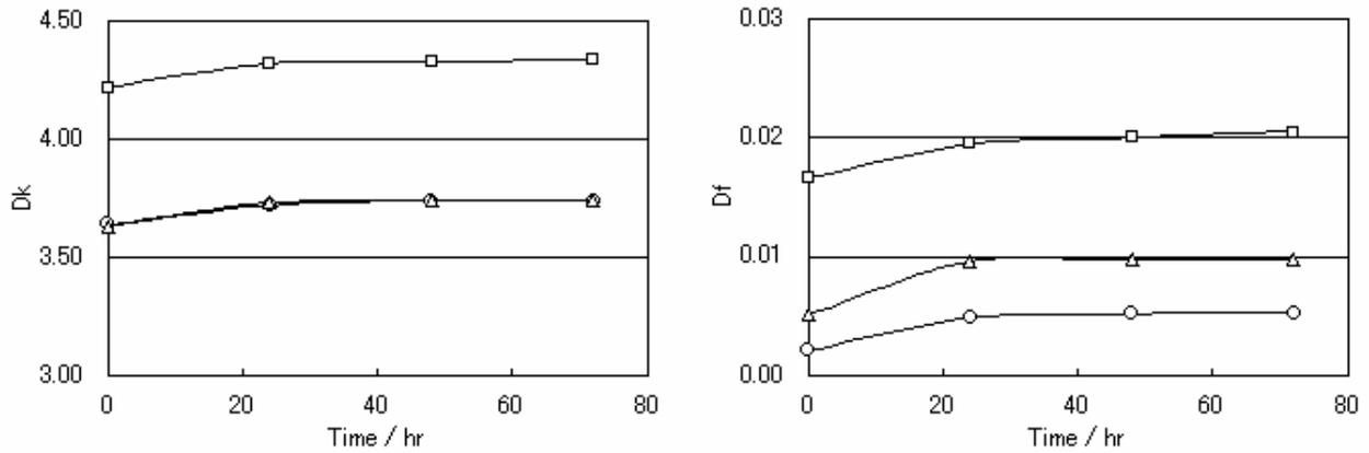
**Figure 3 - The Drifts of Dk and Df with Moisture Absorption - Circle is the Developed Product the Triangle is our Previous Product and the Square is FR-4**
