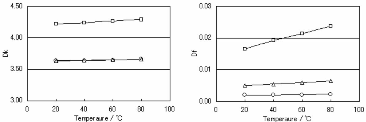
**Figure 2 - Temperature Dependency of Dk and Df - Circle is the Developed Product the Triangle is our previous Product and the Square is FR-4**
