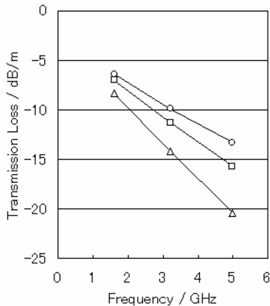
Figure 10 - The Transmission Characteristics results for Various Copper Foils – the Circle is S-VLP Copper Foil, the Square is VLP Foil and the Triangle Is Normal Foil
