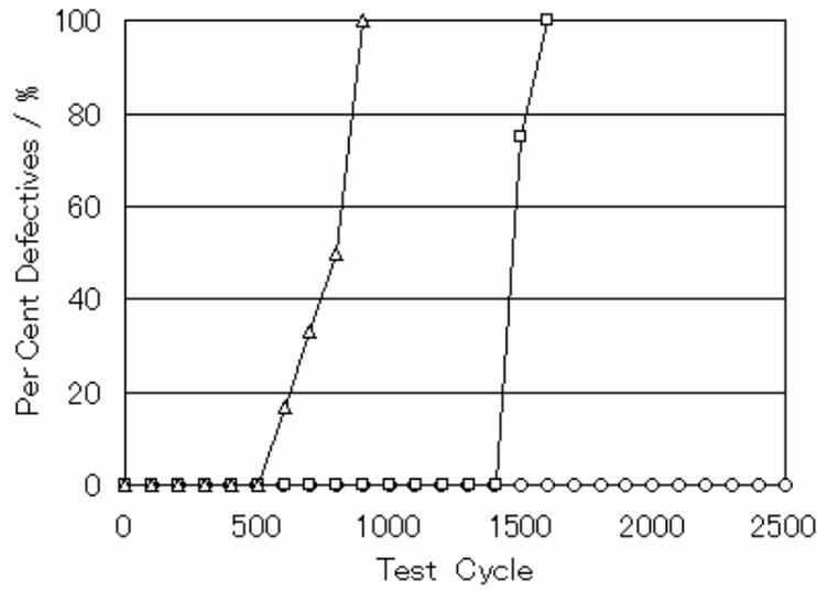
**Figure 6 -The evaluation Results of the Through-Hole Connection Reliability – the Circle is the Developed Product, the Triangle is our Previous Product and the Square is FR-4**
