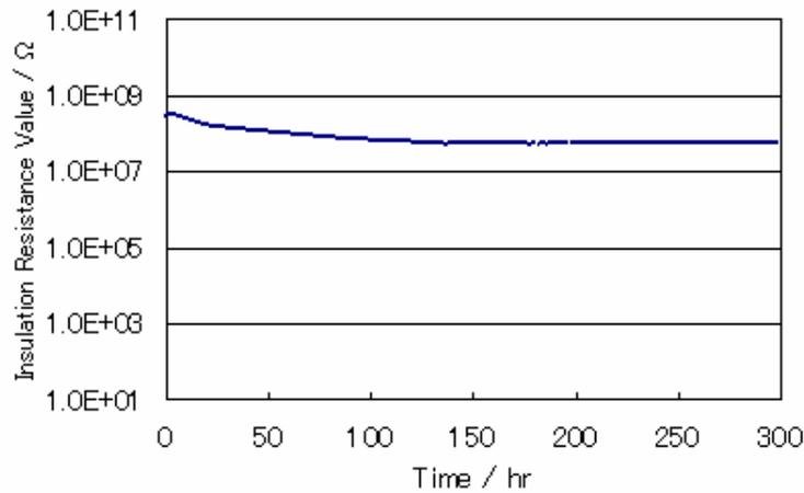
**Figure 8 - Insulation Reliability under the HAST (110°C, 85%, 50V) Conditions**
