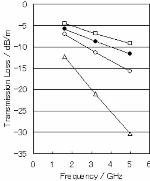
**Figure 11 - Transmission Loss of Various Materials using VLP foil – the Circle is the Developed Product, the Square is our Previous Product and the Triangle is FR-4 - the Closed Circle is the Developed Product using S-VLP Foil and Low-Dk Glass Cloth**
