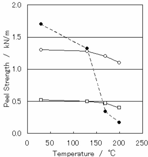
**Figure 4 - Temperature dependency of the copper peel strength - Open Circle is the Developed Product (Normal Copper Foil), the Closed Circle is FR-4 and the Square is Inner-Copper Peel Strength of Developed Product**
