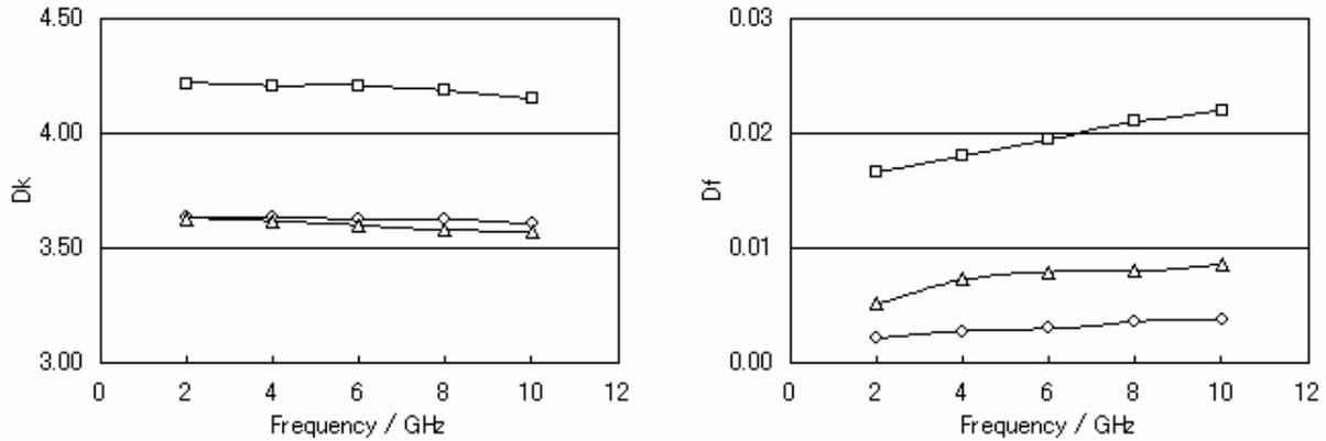
**Figure 1 - Frequency Dependency of the Dielectric Property - The Circle is Developed Product, the Triangle is our previously Developed Product and the Square is FR-4**
