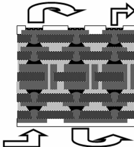
**Figure 7 - Daisy Chain of Specimen**
