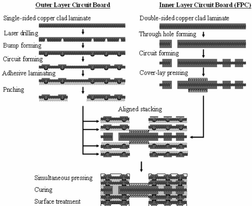
**Figure 2 - Fabrication Process**
