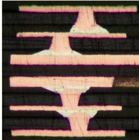
**Figure 6 - Cross Section Photograph of 6-Layered SBic**
