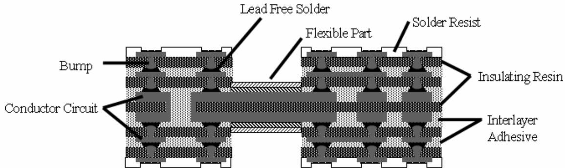
Figure 1 – Schematic Structure (6-layered)
