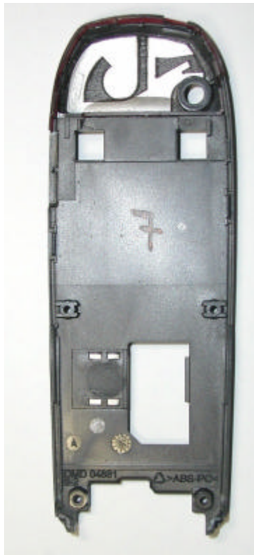
Figure 3 - Polymer Antenna on a Mobile Phone Casing
