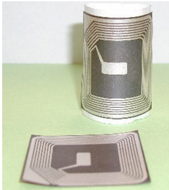
Figure 2 - Flexible Silver Ink on Kapton™ RF Tag
