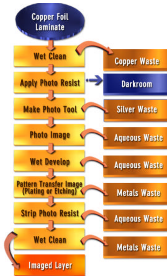
Figure 1 - Sources of Waste in Photolithographic PCB Production
