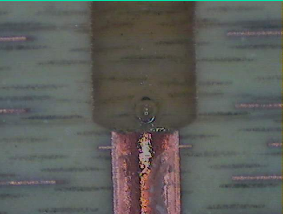
microsection without thermal stress
