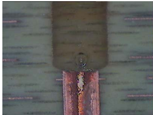
5 - Microsection without Thermal Stress
