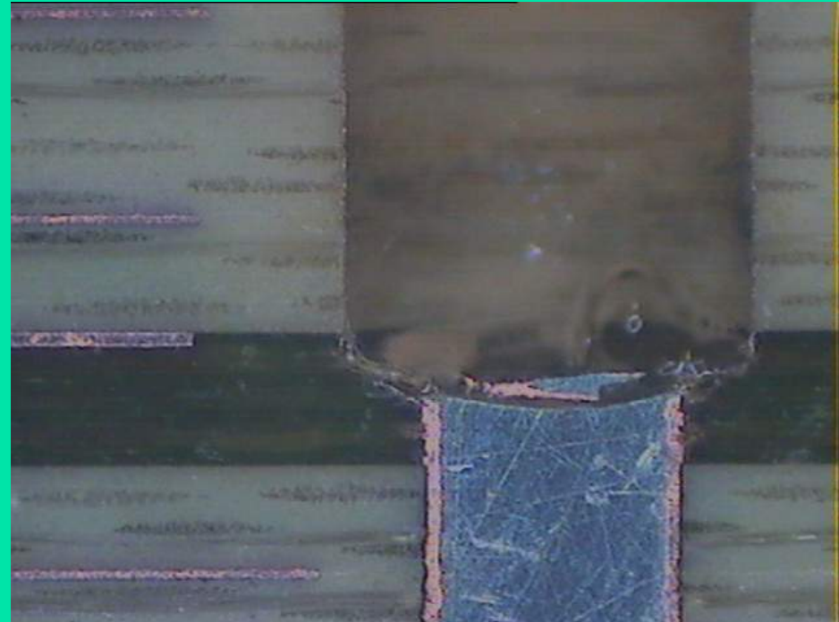
microsection with five times thermal stress
