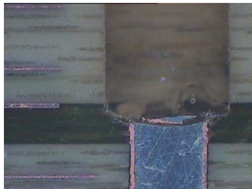
Figure 6 - Micro Section with Five Times Thermal Stress
