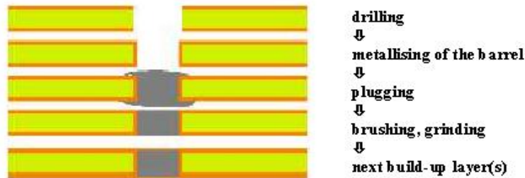
Figure 10 - Process Flow for Applying the Plugging Paste
