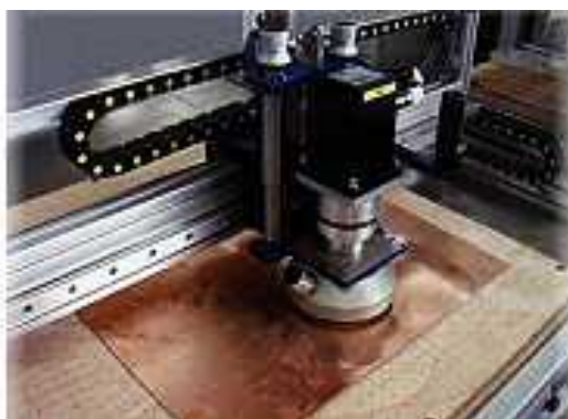
Figure 17 - Orbital Sanding Unit for Planarization of the Inner Layers after Plugging
