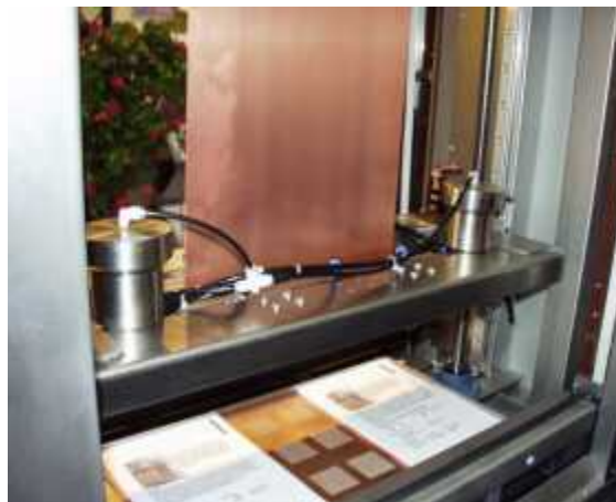
Figure 8 - Vacuum Plugging Machine with Opened Front at the Front the Special Squeegee with Filler Reservoir
