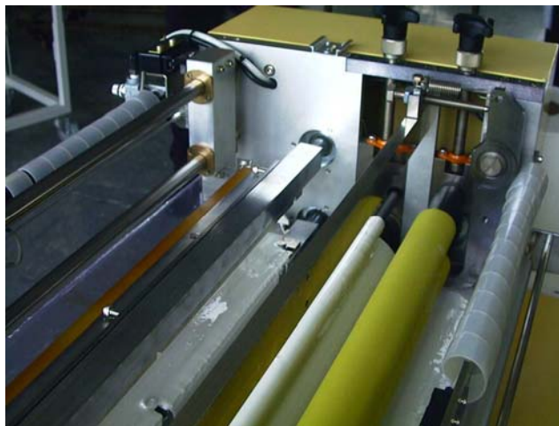
Figure 15 - Plan View of a Roller Coater for the Plugging Process
