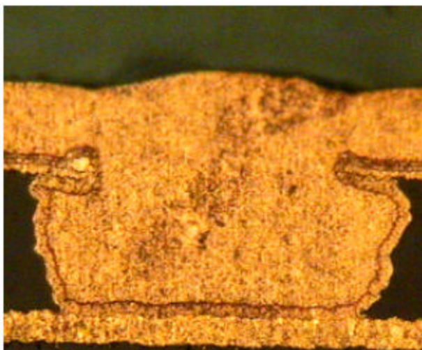
Figure 11 - Copper Metallization of Microvia (Diameter 140 \mu\text{m} ) with Strong Overhang (20 \mu\text{m} )
