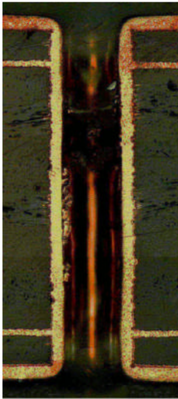
Figure 9 - Through Hole Metallization of Panel Board with PTH > 85 % using an Average Current Density of 1.4 \text{ A/dm}^2 for 100 Minutes (Hole diameter: 0.2 mm)
