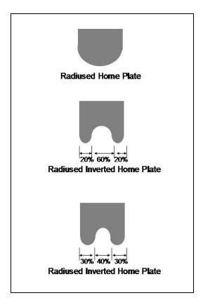
Figure 9 - Experimental Apertures Designed For Lead-Free Paste Printing
