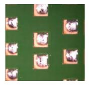
Figure 8 - 0603 and 0805 Pads Before and after Reflow Process (Notice the Lack of Spread)
