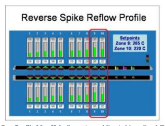
Figure 1 - Reverse Spike Reflow Profile May Help Some Assemblies Achieve Good TALs without Exceeding Peak Temperatures
