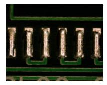
Figure 7 - Lead-Free QFP Print Before And After Reflow (Notice the Lack of Spread during Reflow Process)
