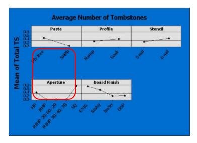
Figure 11 - Tombstone Interaction Plot. Notice All of the Experimental Apertures Minimized Tombstones, but the 20-60-20 Aperture Also Minimized MCSBs
