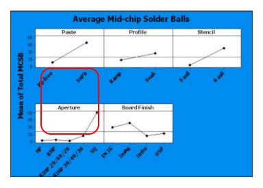
Figure 10 - Mid-Chip Solder Ball Interaction Plot
