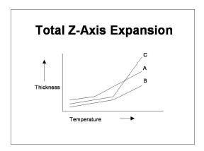
Figure 12 - Expansion of Three Different Base Laminates. Notice that All Post- $T_g$  CTEs are Higher than Pre- $T_g$  CTEs. Material A Exhibits More Total Z-axis Expansion than B Because Of a Lower- $T_g$ , But Material C, Even with a Higher  $T_g$ , Exhibits more Total Z-Axis Expansion than A because it has a High Post- $T_g$  CTE
