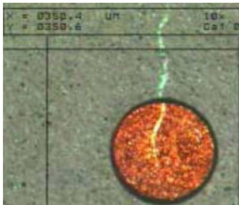
Figure 12 – Example of No laser Alteration of Copper Surface by UV Laser Processing<sup>5</sup>
