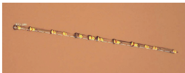
Figure 3 – Pinholes Caused by Mechanical Damage
