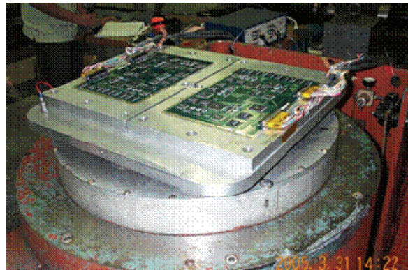
Figure 5 - JG-PP / JCAA Test Vehicle Mounted On Vibration Table
