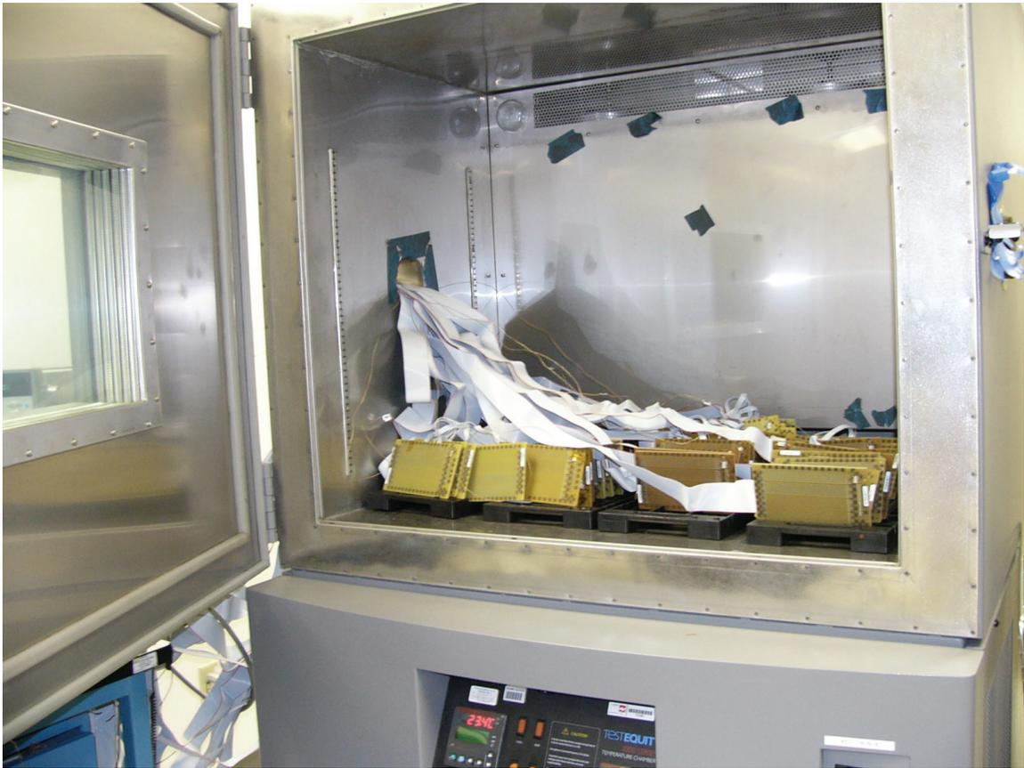
**Figure 5 - Test Boards in The Thermal Cycle Chamber**
