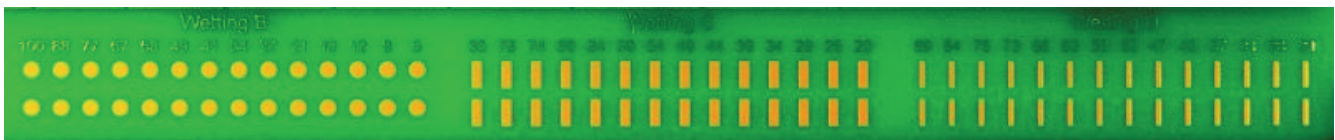
Figure 1 - Spread test areas on Benchmark II Test Board
