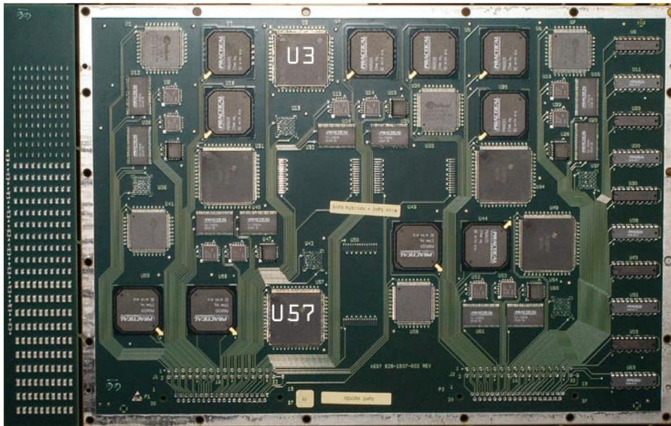
Figure 31 - Locations of U3 and U57 Reworked TQFP-208 Components
