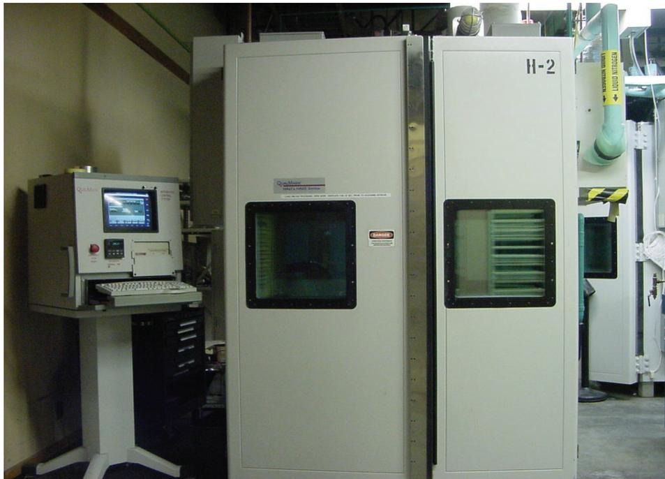
**Figure 1 - Qualmark Model OVS-4 HALT/HASS Chamber**
