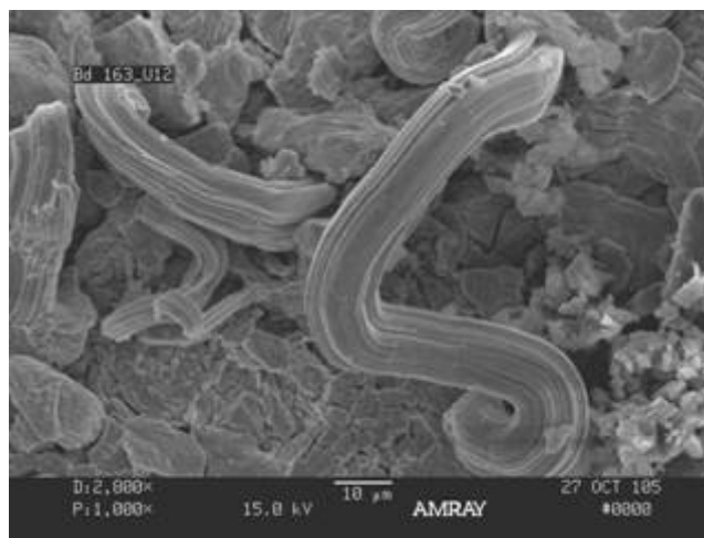
Figure 12. High magnification SEM image of TSOP component with SnCu surface finish showing individual tin whisker on upper knee of lead (Component U12, test vehicle 163)
