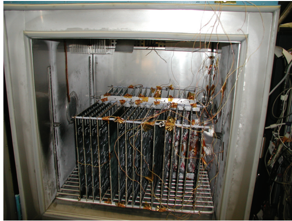
Figure 4. Test vehicles loaded into the -55°C to +125°C test chamber.
